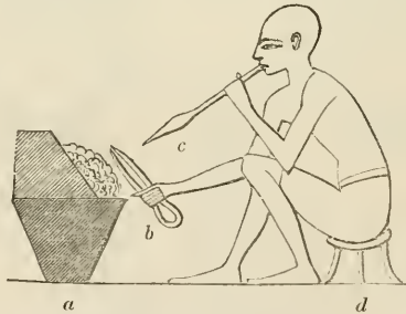
No. 375. Blowpipe, and small fireplace with cheeks to confine and reflect the heat. Thebes .
