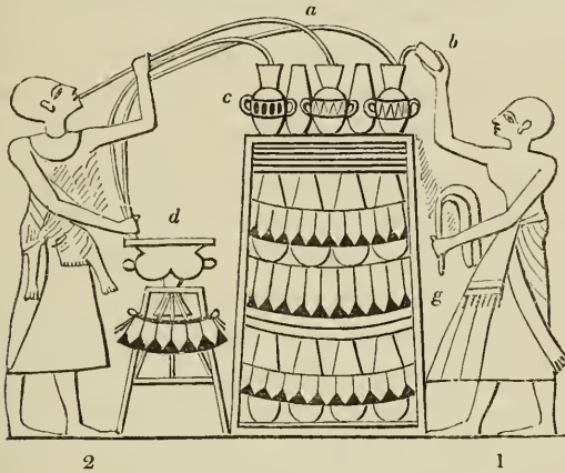
No. 394. Siphons used in the year 1450 B. C. Thebes. 1 pours a liquid into vases from the cup b ; and 2 draws it off by the siphons a .
