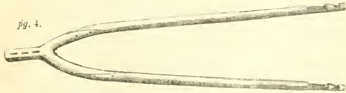
Fig. 1. Wheel; 3 ft. 1 in. diameter. Fig. 4. Shafts; 11 feet in total length.
