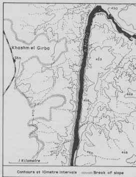
FIG. 83. The Atbara gorge at Khashm el Girba. The Arabic term means literally "the mouth of the water skin"; this is the site where a dam may come to be built to command about 500,000 feddans on the west bank of the river (Fig. 82). From Irrigation by gravity from the River Atbara , 1955, Fig. 4, Sheet 1.
