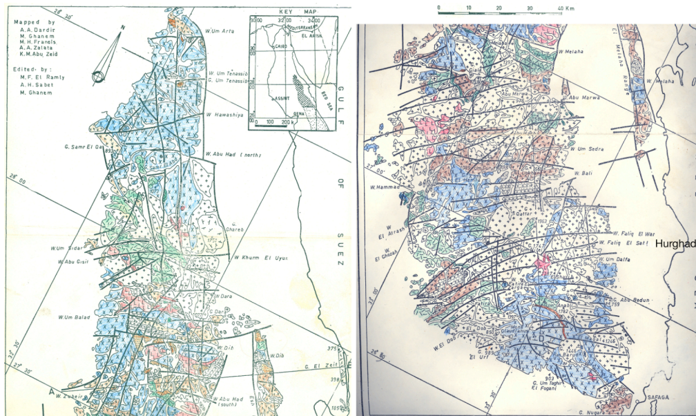
Fig. 45: Geologic map of the NE Desert, from (Ghanem et al., 1973). Granodiorites are blue 'X's, younger granites are white '+', Dokhan volcanics are brown 'v's, metavolcanics of unknown age are green lines, gabbros are red 'L's.
