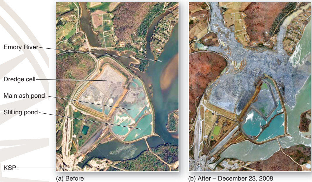
FIGURE GN 13.1 Before and after the TVA ash slurry spill disaster.
