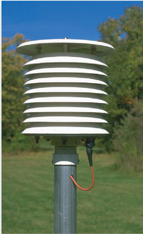
FIGURE 5.3 Instrument shelter. This standard thermometer shelter is white and louvered, installed above a turf surface. These are replacing the traditional Cotton-region, or Stephenson screen, shelters for temperature measurement. [Bobbé Christopherson.]
