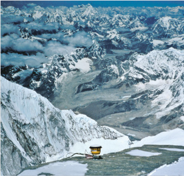
FIGURE 1.20 GPS used to measure Everest's summit height. Installation of a Trimble 4800 GPS unit at Earth's highest benchmark, only 18 m (60 ft) below the 8850-m (29,035-ft) summit. Previously, the height was set at 8848 m. Scientists using GPS data accurately analyzed the rate the mountain range is moving due to tectonic forces. [Photo and GPS installation by adventurer/climber Wally Berg, May 20, 1998.]
