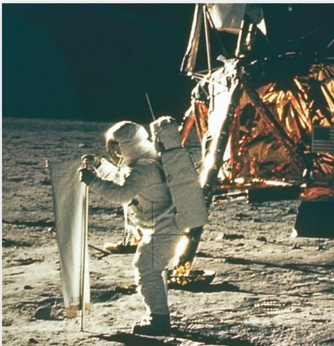
FIGURE 2.3 Astronaut and solar wind experiment. Without a protective atmosphere, the lunar surface receives solar wind charged particles and all the Sun's electromagnetic radiation. An Apollo XI astronaut in 1969 deploys a sheet of foil in the solar wind experiment. Earth-bound scientists analyzed the foil upon the astronauts' return. Why wouldn't this experiment work if we set it up on Earth's surface? [NASA.]
