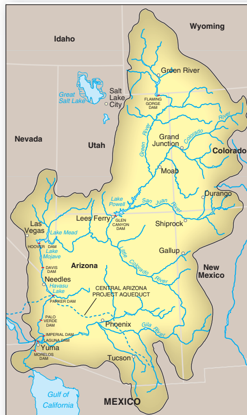
FIGURE GN 9.1 The Colorado River Basin. The region is divided between an Upper Basin and a Lower Basin. The river from 1990 to 2009 averaged only 11.20 maf (million acre feet) of discharge per year. In its water budget, inputs do not equal outputs and the reservoirs are declining.
