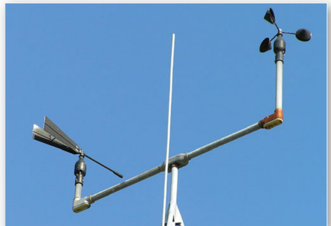
FIGURE 6.4 Wind vane and anemometer. Instruments used to measure wind direction (wind vane, left) and wind speed (anemometer, right) at a weather station installation. [NOAA Photo Library.]
