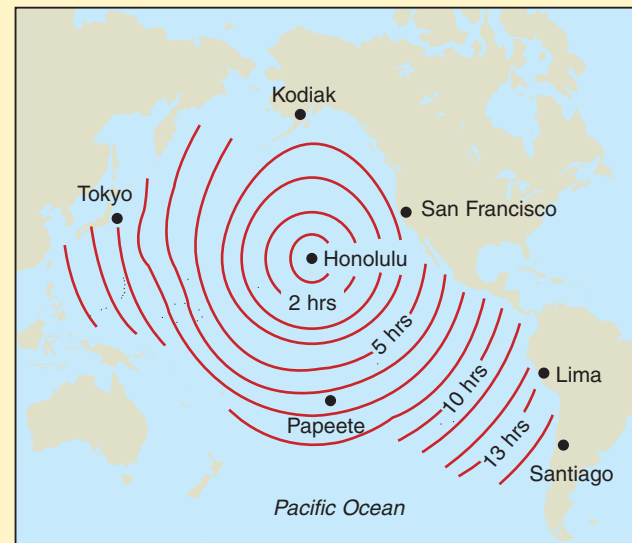
The PTWC locates earthquake epicenters and estimates times of arrival for potential tsunamis in the Pacific region.
