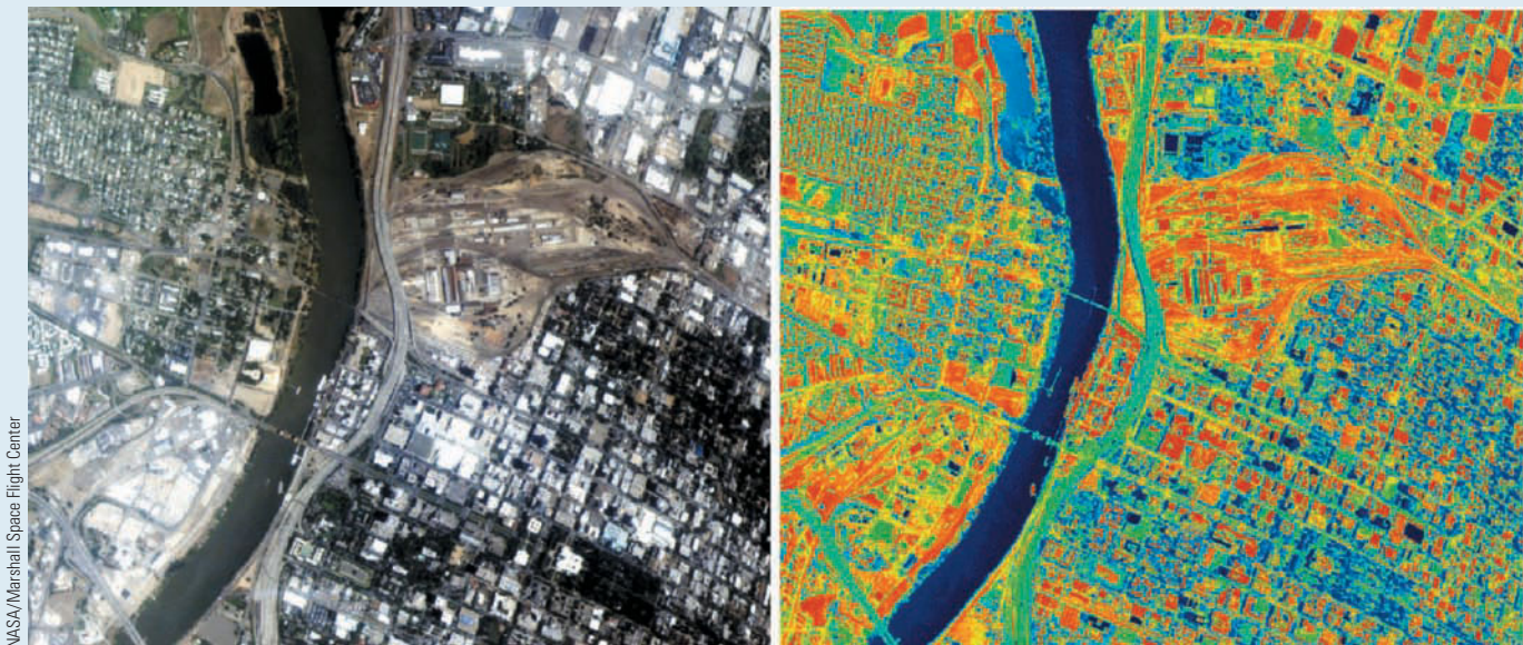
The urban heat island effect in Sacramento, California. The thermal image (right) shows the heat retention of buildings and densely urbanized areas at night. The hottest areas are in red, less hot areas in yellow or green, and cooler areas in blue, like the Sacramento River, parks, and neighborhoods (which are cooled by the presence of trees). Comparing sections of the thermal image to the aerial photograph (left) illustrates the relationships between built-up areas, vegetated areas, water bodies, and their relative temperatures at night.
