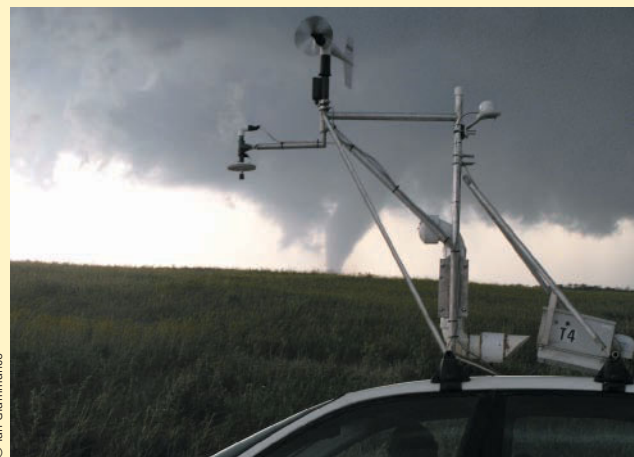
Scientists who “chase” tornadoes seek to observe them from as near as is safely possible, in order to gain important information to help us understand how these storms function. With a large tornado in the background, this vehicle is mounted with special equipment for tornado tracking and data gathering.
