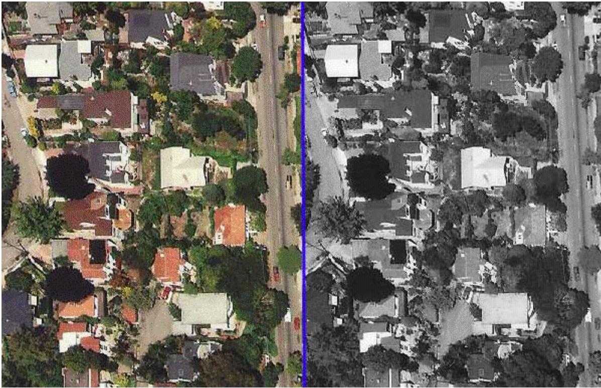
{PRIVATE}Figure 2e -2: Comparison of black and white and color images of the same scene. Note how the increased number of tones found on the color image make the scene much easier to interpret. (Source: University of California at Berkeley - Earth Sciences and Map Library ).
