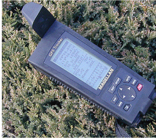
{PRIVATE} Figure 2b-11: Handheld Global Positioning Systems (GPS). GPS receivers can determine latitude, longitude, and elevation anywhere on or above the Earth's surface from signals transmitted by a number of satellites. These units can also be used to determine direction, distance traveled, and determine routes of travel in field situations.
