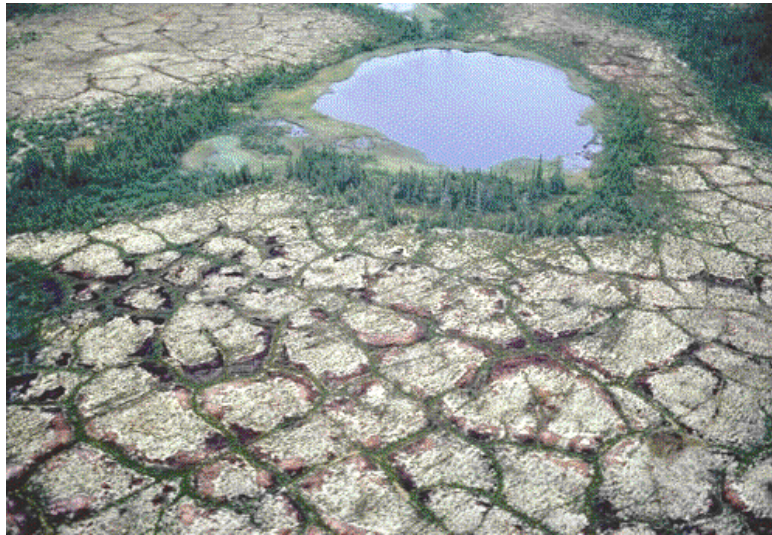
{PRIVATE} Figure 11q-7: Ice-wedge polygons in peatland, Hudson Bay Lowlands, Manitoba. Splendid examples of ice-wedge polygons, a form of patterned ground, are shown above. They occur in the permafrost peatlands of the Hudson Bay Lowlands, which are composed mainly of dry sphagnum. Brown polygons mark the location of massive ice wedges that extend from the surface down to 2 or 3 m. (Source: Natural Resources Canada - Terrain Sciences Division - Canadian Landscapes ).
