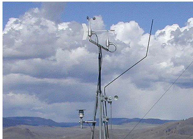
{PRIVATE} Figure 7n-2: Meteorological instruments used to measure wind speed and direction. Wind speed is commonly measured with an anemometer . An anemometer consists of three open cups attached to a rotating spindle.
