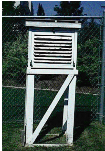
{PRIVATE} Figure 7k-1: Well ventilated instrument shelters are used to protect thermometers from precipitation, direct sun, and other physical elements. Construction standardization of these shelters, by international agreement, guarantees that measurements are comparable in any of the over 15,000 weather stations found worldwide.
