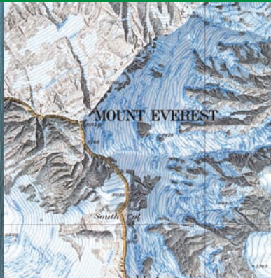
▲ A topographic map of Mount Everest combining topographic contours with shaded relief.
