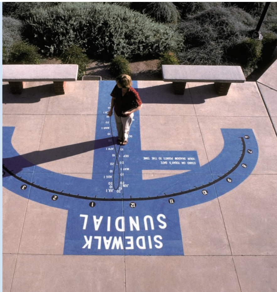
B This version of a sundial at the University of Arizona is a solar timekeeper. The user selects a standing position based on the day of the year and reads the time from his or her shadow.
