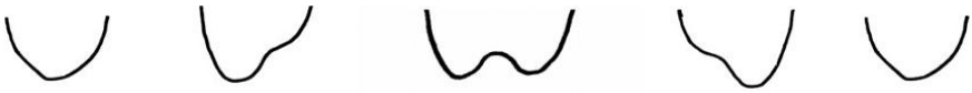
Figure 5.6. Variation of the potential function (vertical section in Figure 5.5). In the center: two minimum stable and one maximum unstable, corresponding to the shaded area of Figure 5.5
