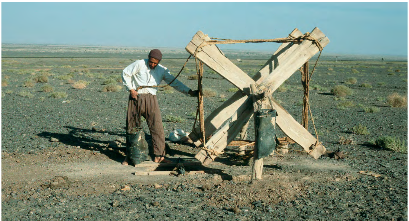
Fig. 6 & 7: Oriental turning-cross winch above a qanat-shaft near Rafsandjan. Each turn brings up as much as 4 m of rope. The winch can easily be taken apart for transport; Photo: G. Weisgerber 1978.
