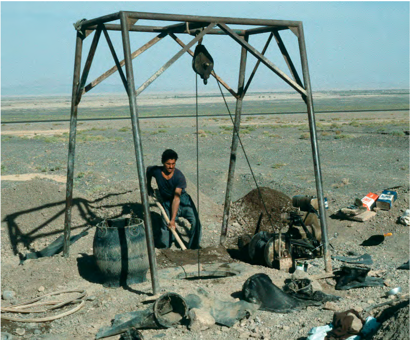
Fig. 8: Modern winch-scaffold with petrol-driven engine and a hoisting bucket made of old lorry-tyres near Rafсанджан; Photo: G. Weisgerber 1978.
