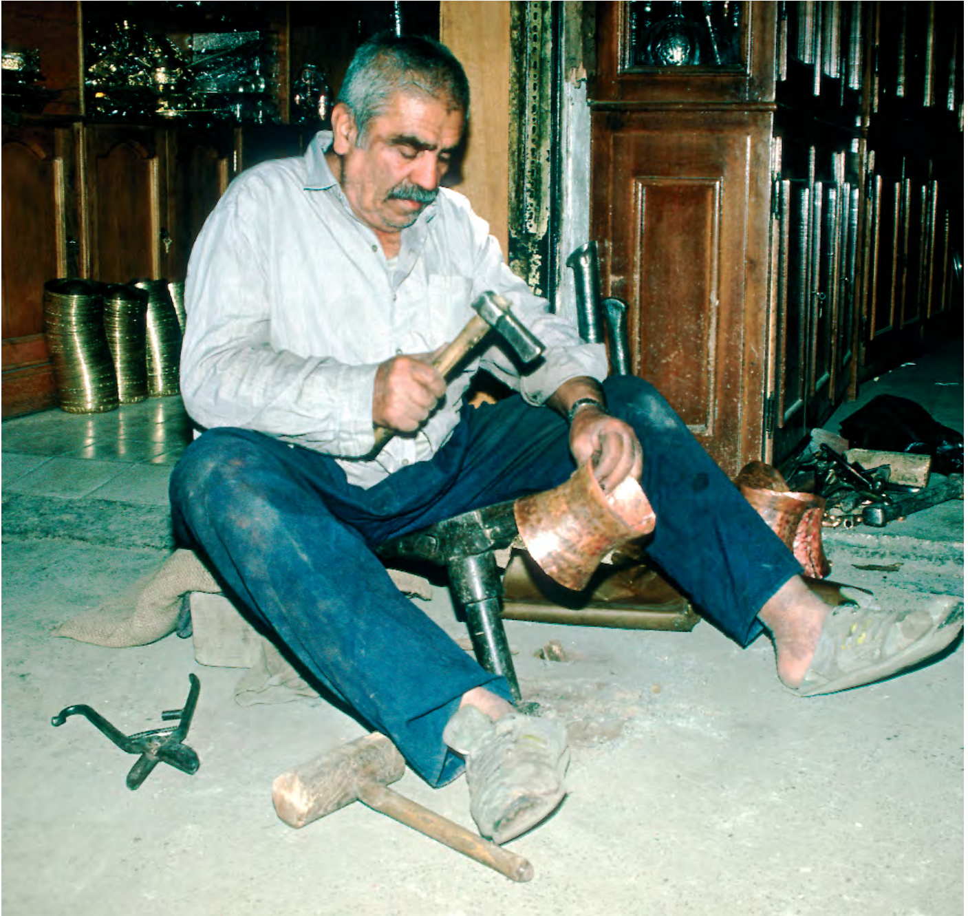
Copper smith in the bazaar of Isfahan, driving a beak shaped workpiece (2000); Photo: Th. Stöllner.
