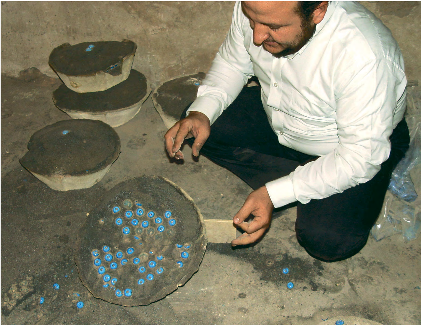
Fig. 7: Opening the vessels after cooling down. The blue beads are clearly visible in the grey powder.
