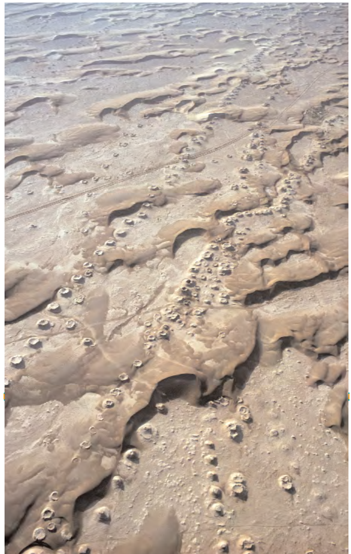
Fig. 1: On desert terrain, several generations of ring-shaped heaps from qanat-shafts are visible. Several lines mean several periods of construction. Like in the case of the two long lines this may be a new construction or, like the two shorter lines, they may be extensions or only repairs of broken drifts; Photo: Georg Gerster.
