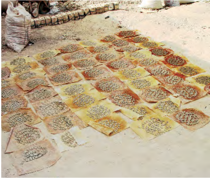
Fig. 4: In the court the wet basic shapes are laid out for drying.
