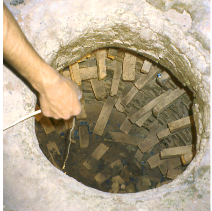
Fig. 6: Empty kiln, 2.5 m deep. The vessels are stacked in between the ceramic spacers.
