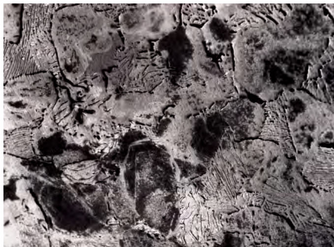
Fig. 3: Photomicrograph of iron sword UM 65-31-220, showing pseudomorphic pearlite colonies (note their lamellar structure) preserved in the oxidized matrix of the sword. The light coloured, elongate lamellae are probably uncorroded carbides. This artefact had evidence of evenly distributed carburization (in the form of pearlite colonies) in the central portion of the blade, as well as at the blade's edge. Thus it would qualify as a "mild" steel and most probably was an effective weapon of war. Along one edge of the blade distorted structures in the oxide suggest some evidence of cold-working deformation of the metal. Grain size, when apparent, is seen to be coarse, and there is some indication of the artefact having been cooled fairly slowly (Pigott 1989, 76, Fig. 15).
