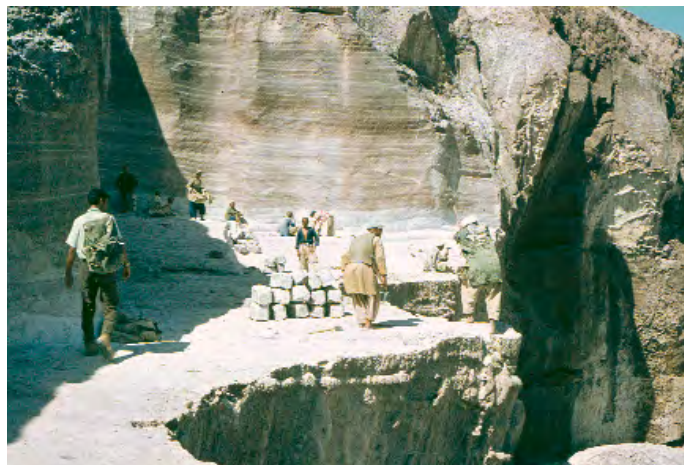
Fig. 3: Salt-quarrying at the Taqcha Khana-diapir. A new bank is opened up after the residual clay (on the right) has been removed. The view is WSW across the Rod e Namakab-canyon and to the small western part of the salt-deposit. Photo: August 1970 (slides-archive H. K. 2422).
