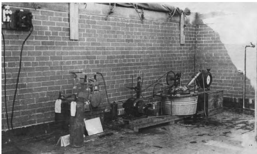
7. Apparatus first used to produce lewisite at Catholic University of America, ca. 1918. Note the washbasin, which probably served as a cooling bath. Also note the air tanks, which were probably filled with acetylene. Courtesy Philip Reiss.
