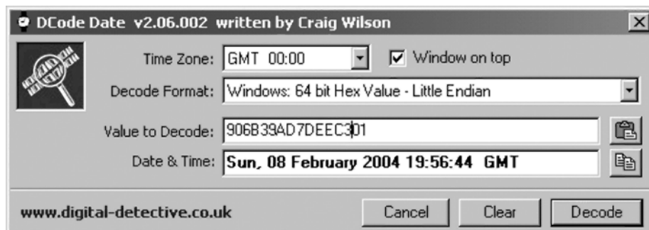
Figure 11.8 DCode used to convert 64-bit FILETIME date- time stamps from their hexadecimal representation
