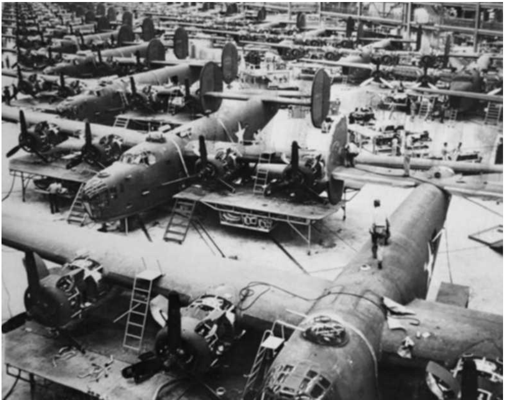
Below: President Roosevelt's great arsenal of democracy in action: seemingly endless B-24 Liberator bombers on the assembly line at the Ford Willow Run plant in Detroit, Michigan
