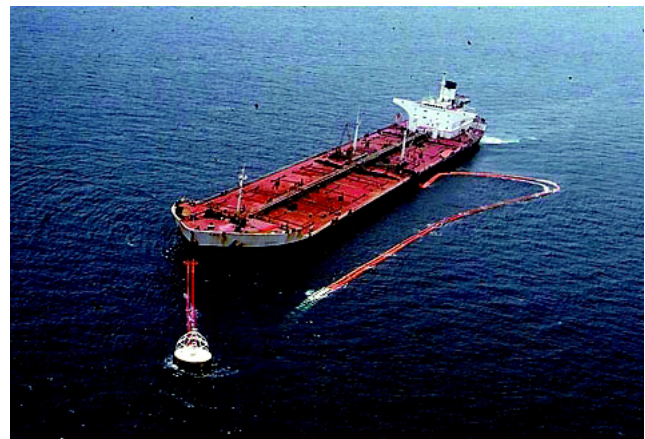
PHOTO 3 Lightering oil from a supertanker at the Louisiana Offshore Oil Port in the Gulf of Mexico south of New Orleans. Tankers have historically been seen as a major source of oil pollution. Recent changes in tanker design (e.g., introduction of partitioned tanks and double hulls) and in oil handling procedures (e.g., offshore lightering) have significantly reduced the size and frequency of spills (Photo courtesy of Nancy Rabalias.)
