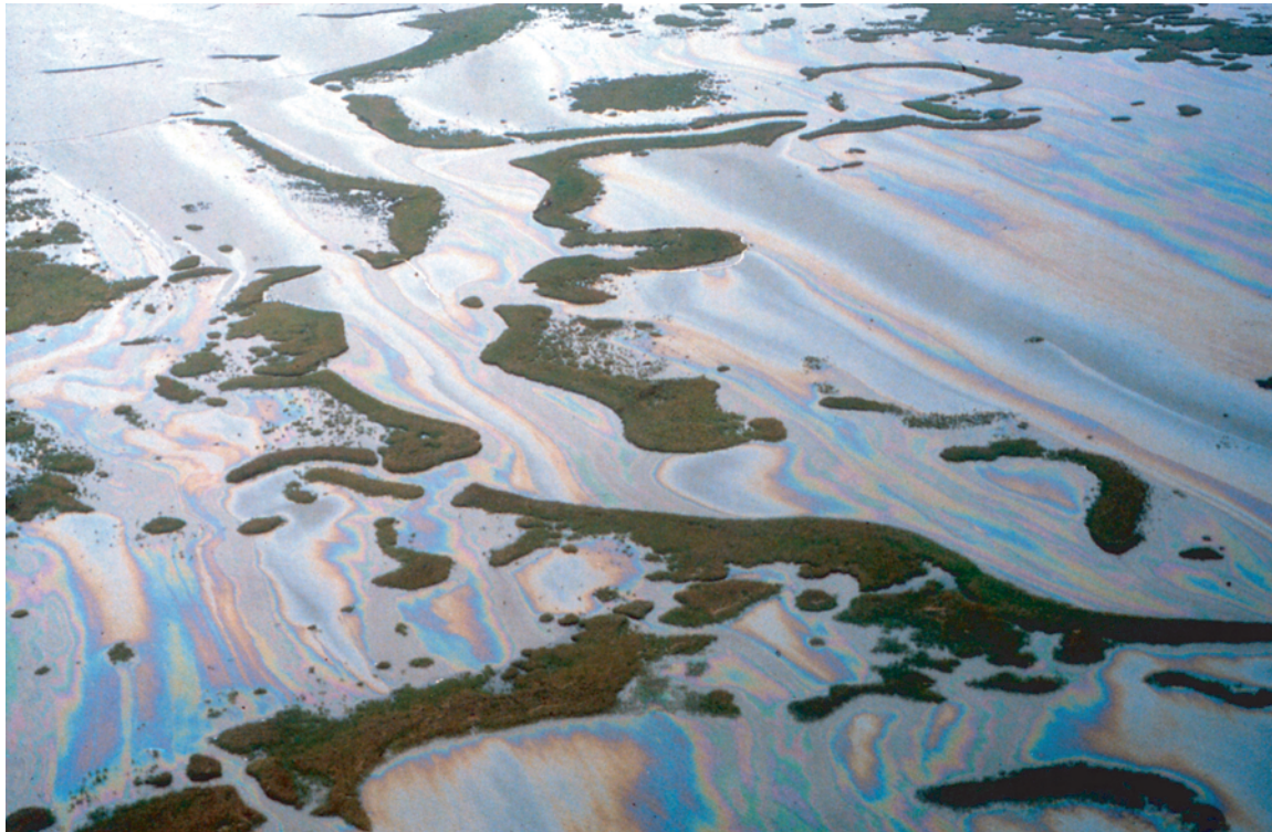
PHOTO 16 A spill of roughly 320,000 gallons of south Louisiana crude in May 1997, streaming across the broken marshes of Lake Barre. There is very little substrate exposed thus the oil is being pushed through the submerged vegetation by wind. (Photo courtesy of Jacqui Michel, Research Planning, Inc.)
