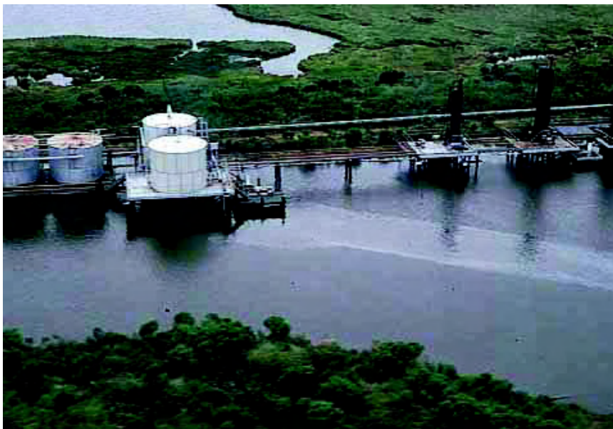
PHOTO 8 Even a relatively small spill (one gallon) can generate a visible slick that extends for some distance from the source. Additional research is needed to evaluate the cumulative impact of such small releases that occur regularly in a given area, especially when they occur in sensitive areas such as coastal wetlands. (Photo courtesy of Nancy Rabalais.)
