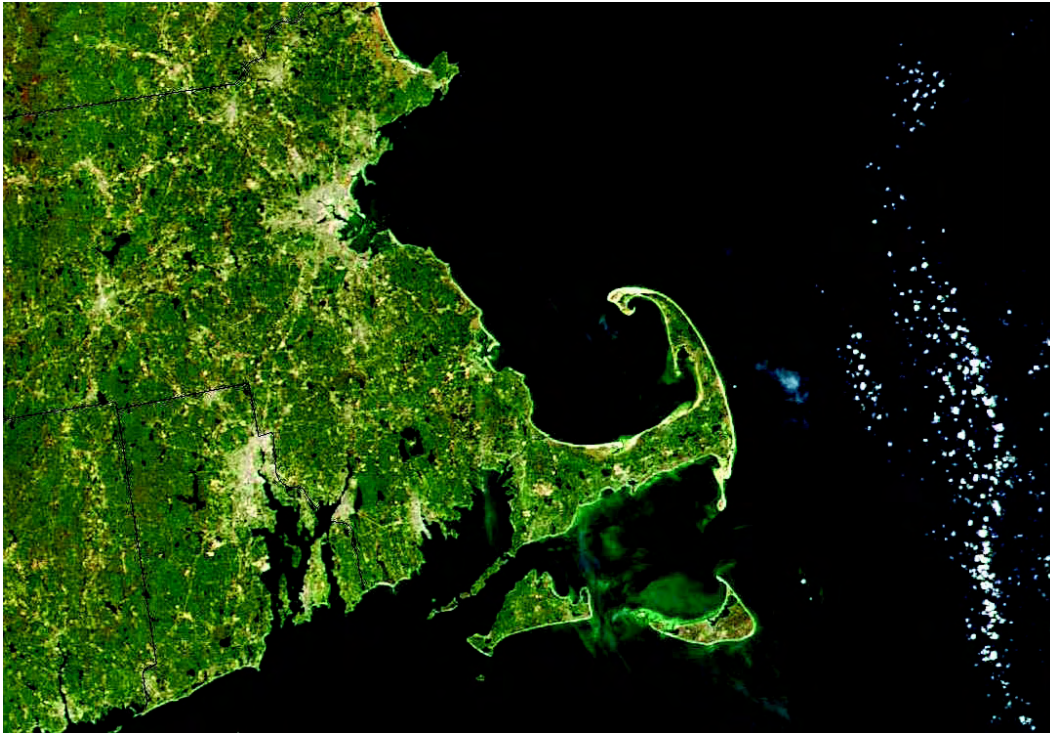
PHOTO 22 MODIS (or Moderate Resolution Imaging Spectroradiometer) satellite imagery (250 m resolution) of New England. Urbanization, visible from space, increases both population density and the percent of paved surface, altering the volume and composition of runoff. (Image courtesy of NASA.)
