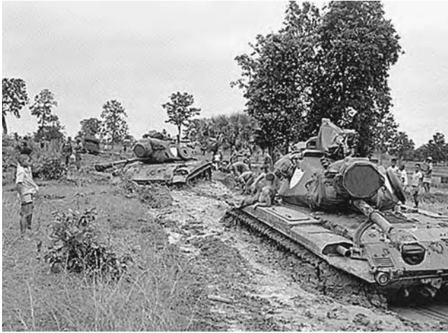
The U.S. Army often found itself poorly equipped for fighting conditions in Vietnam, as these two M-41 tanks, mired in the mud of a monsoon, attest. Collection: National Archives and Records Administration
