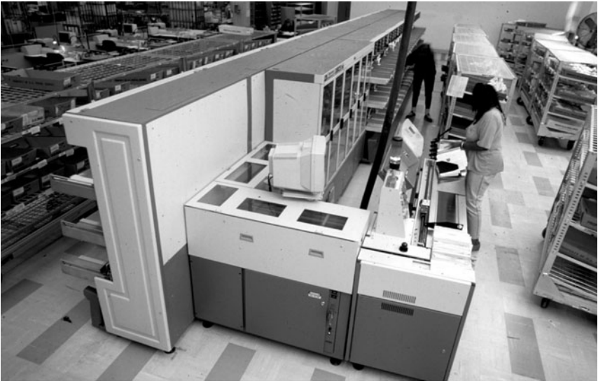
Twenty-first-century equipment. Two people operate a delivery barcode sorter, one feeding in stacks of letters, the other “sweeping” sorted letters into trays in delivery order. © 1992 U.S. Postal Service. All rights reserved. Used with permission.
