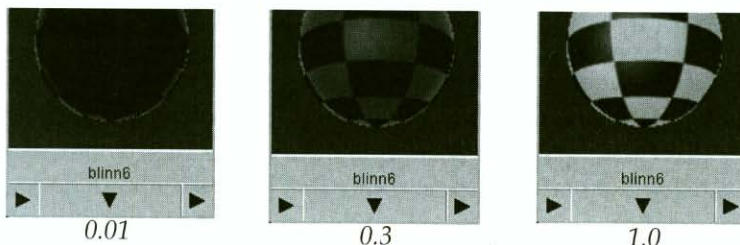
Effect of Specular Roll Off on Reflectivity (Reflected Color mapped with checker)
