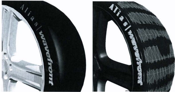
Displacement to Polygon Tool results
