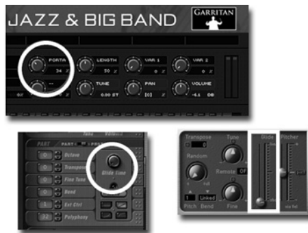
Figure 4.26 Portamento parameter in the ESX24, Mach5, and Garritan Jazz and Big Band library (Courtesy of MOTU, Garritan, and Apple Inc).
