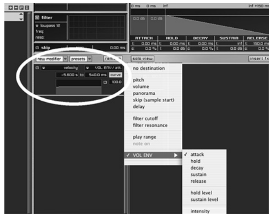
Figure 5.17 In Independence any modifier (CCs, MIDI Data, etc.) can be assigned to virtually any parameter of a patch. In this case MIDI velocity was assigned to the attack section of the volume (amplifier) envelope (Courtesy of Yellow Tools).
