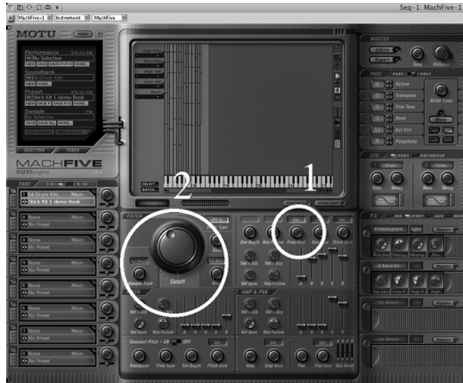
Figure 2.26 Example of velocity-controlled filter in MOTU MachFive where MIDI velocity (1) is set to control the cut-off frequency of a low pass filter (2) (Courtesy of MOTU).
