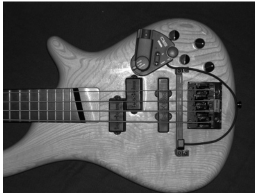
Figure 2.16 A Yamaha bass to MIDI converter in the 4 strings configuration (Courtesy of Yamaha).
