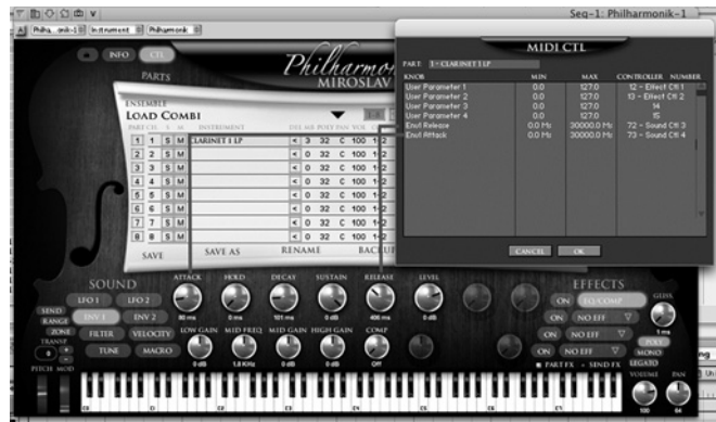
Figure 4.27 Example of CC#72 and CC#73, the release and attack of a clarinet patch in IK-Multimedia Philharmonic (Courtesy of IK-Multimedia).
