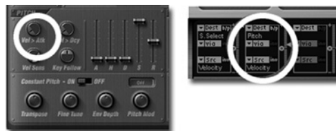
Figure 4.28 Two examples of velocity to tuning assignment: MOTU MachFive and Apple EXS-24 (Courtesy of MOTU and Apple Inc).
