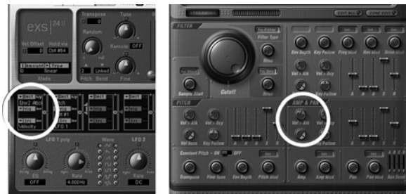
Figure 4.24 Example of an amplifier envelope controlled by the attack velocity in the EXS24 and Mach5 software samplers (Courtesy of MOTU and Apple Inc).
