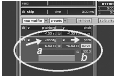
Figure 5.24 Example of MIDI velocity applied to pitch control. Notice how in this case you can determine (a) the overall amount of detuning and (b) the curvature of the variation (Courtesy of Yellow Tools).
