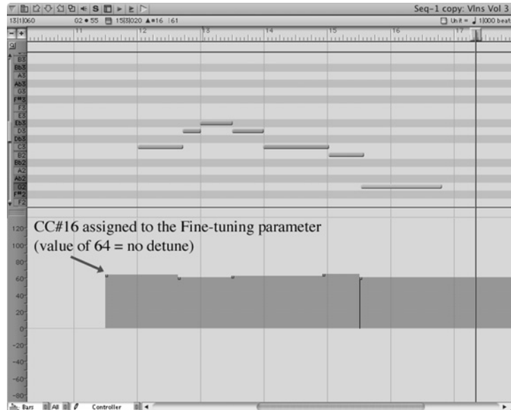
Figure 3.39 Example of horizontal detuning applied to a viola section. CC#16 was assigned to the fine-tune parameters of the patch and subtle variations were penciled in along the part (Courtesy of MOTU).
