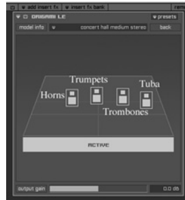
Figure 5.32 Positioning of the brass instruments for the symphony orchestra using the Origami LE convolution reverb by Yellow Tools (Courtesy of Yellow Tools).
