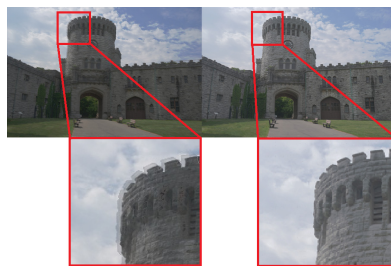
Fig. 1. Effects of motion compensation: the left one is synthesized directly without motion compensation while the right one is synthesized after relatively accurate motion compensation
