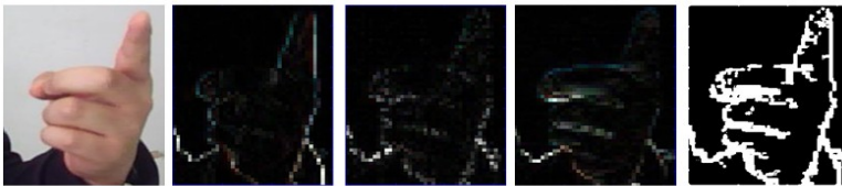
Fig. 2. Extraction of edges based on the WMT. Original image, edge image of vertical components, edge image of horizontal components, edge image of diagonal components, combination of the three components from left to right, respectively.
