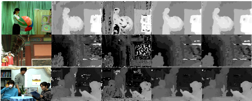
Fig. 4. Comparison of initial and refined depth maps. From the first column to the last column are original images, our initial results, results in [3], our refined results and the results of joint-trilateral filter, respectively.
