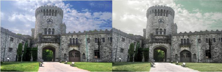
Fig. 2. Color HDR image synthesized in different color space. The left one is synthesized in RGB color space, while the heavily distorted one on the right is synthesized in HSI color space.
