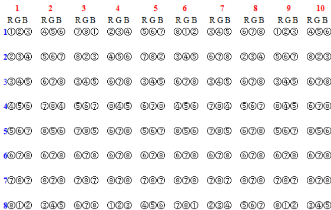
Fig. 2. Synthesized diagram of 8-view stereo display
