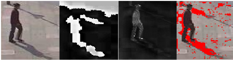
Fig. 2. Some results of shadow suppression. Original image, H component, S component and detected shadow results (marked as red color), from left to right, respectively.
