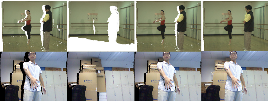
Fig. 5. Experimental Results (in turn from left to right): The image after mapping; the estimated background; the image after background filling; the image after the second inpainting
