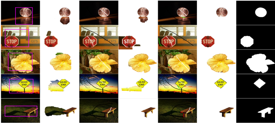
Fig. 5. Segmentation comparison of GrabCut, IAGC and our approach. From the 1 st to the 6 th column: input images with user-specified rectangles and scribbles, and interactive object segmentation results obtained using GrabCut, IAGC and our approach, respectively. The ground truths are shown in the rightmost column.
