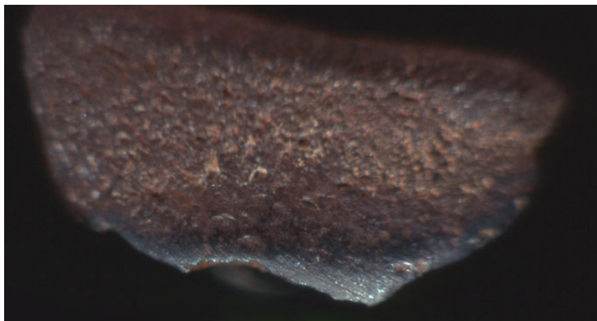
PLATE 4.6 CF Hematite, 1.5g, 21.6 mm length. NCS streak 5030 Y80R. Ground on part of one main surface and two edges, illustrated facet 3.2 mm wide.
