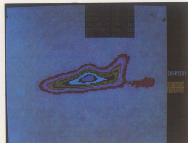
Z-scale Contour of infrared copy print with band pass filtering — topographical view based upon illumination; blue is profile edge of wing closest to camera; shows rear edge (red) slightly larger than front edge due to blurr factor, proving movement of jet; jet exhaust visible, amplified by infrared. ◆ ▲ ■ ● 1. 4. 5.
