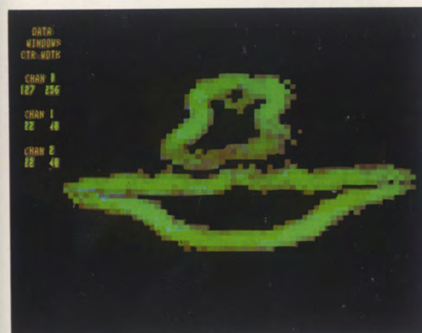
Edge Identification — fighter and spacecraft; eliminates strings, wires, paste-ups, small models due to computer size/distance calculations.
