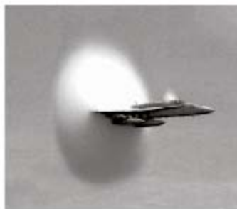
Figure 5.8. Vapor cloud around an F/A-18 jet fighter flying at transonic speed. (U.S. Navy photo by Ensign John Gay)
