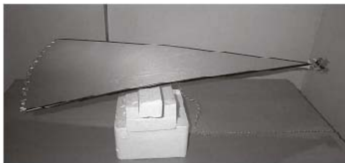
Figure 11.3. A wedge-shaped printed circuit board constructed by Naudin as a test of Dimitriou's experiment. (Courtesy of J.-L. Naudin, from his website, http://jnaudin.free.fr/ )
