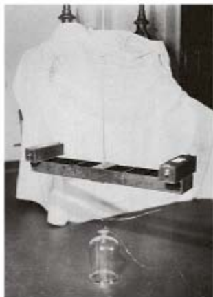
Figure 1.3. An experimental setup designed to measure the thrust produced by Thomas Townsend Brown's gravitators. (Photo courtesy of the Townsend Brown Family and Qualight, L.L.C.)
