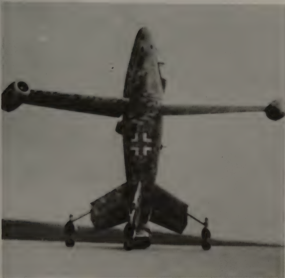
The Focke-Wulf powered wing design, powered by threeLorin ramjet engines. The required initial velocity was to be provided by rockets mounted in the engines.
