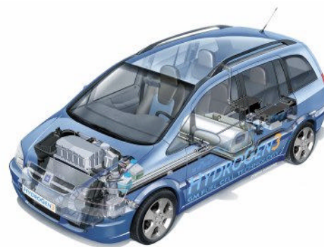
Figure 8-20: Hydrogen powered fuel cell vehicle based on the 'Zafira' platform by General Motors (Opel); the HydroGen3 was built in two versions: with a liquid and a gaseous hydrogen storage tank placed underneath the backseat
