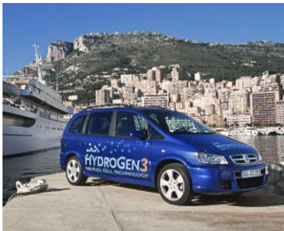
Figure 8-20: Hydrogen powered fuel cell vehicle based on the 'Zafira' platform by General Motors (Opel); the HydroGen3 was built in two versions: with a liquid and a gaseous hydrogen storage tank placed underneath the backseat
