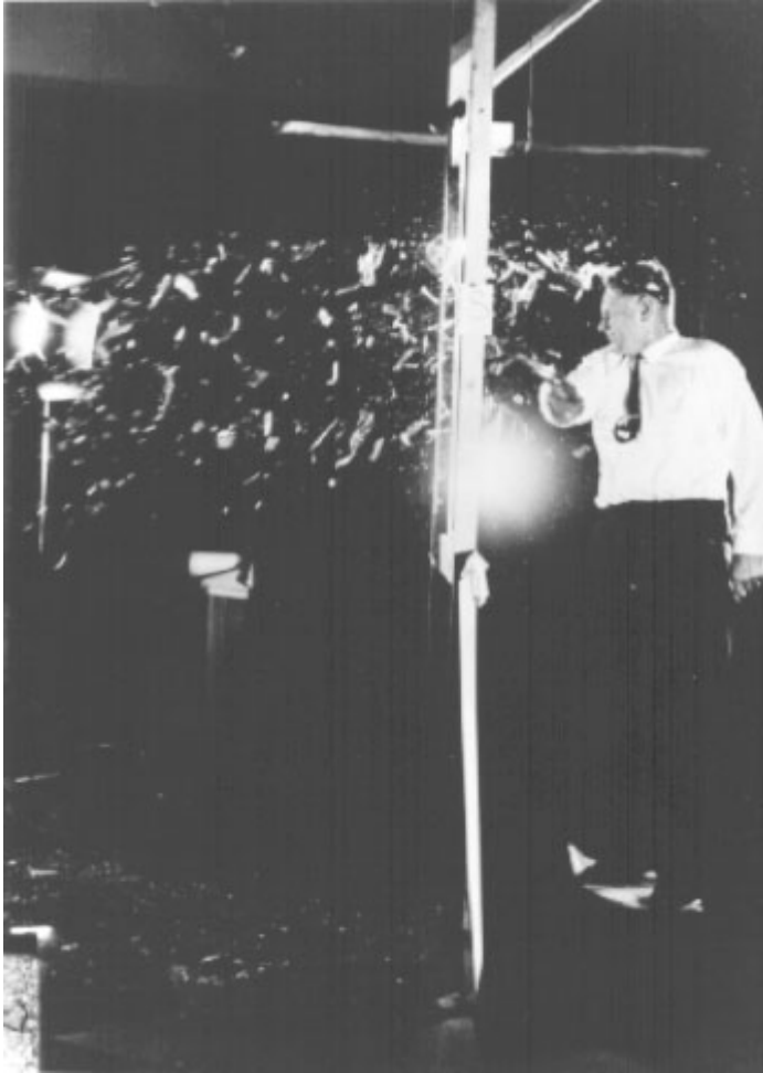
D.F. Nelson and B.C. Revell, Backward fragmentation from breaking glass, J. Forensic Sci. Soc. , 7, 58, 1967 (Reprinted with the kind permission of the Forensic Science Society).
