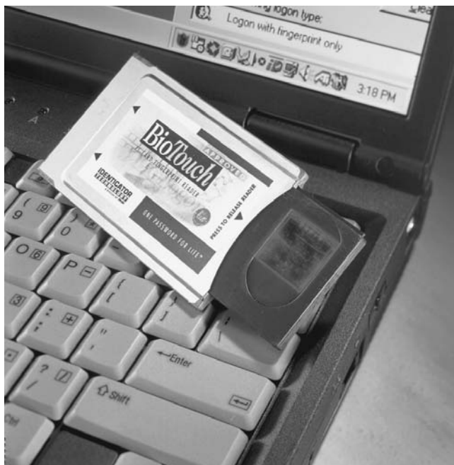
The BioTouch PC Card features an optical fingerprint reader, allowing secure access for laptop users. (Identix Inc.)
