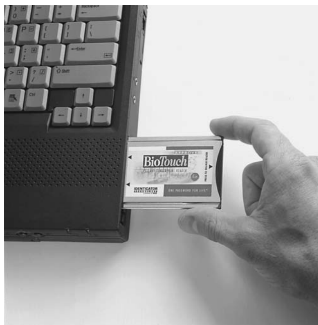
The BioTouch PC Card features an optical fingerprint reader, allowing secure access for laptop users. (Identix Inc.)
