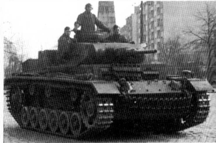
Plates 195-196. Pz Kpfw III Ausf H. A new type of drive sprocket, with six D-shaped holes and open eight-spoked rear idler, was introduced with this model. Note the 30mm armour plates bolted on to the upper and lower nose plates. Above: in Sofia, 1941; below, at speed in North Africa.
