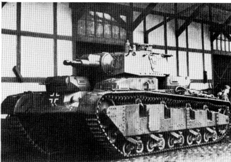
Plate 491. The mild steel Neubaufahrzeug prototype, with Rheinmetall turret mounting the 3.7cm gun above the 7.5cm.
