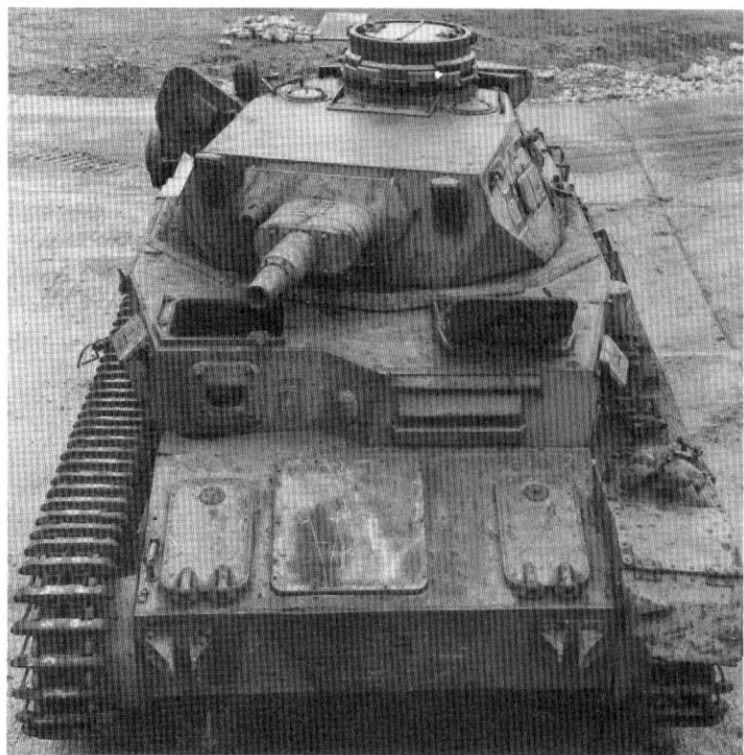
Plate 286. Pz Kpfw IV Ausf D. Note that the hull machine-gun position has been re-introduced within the Kugelblende 30.
