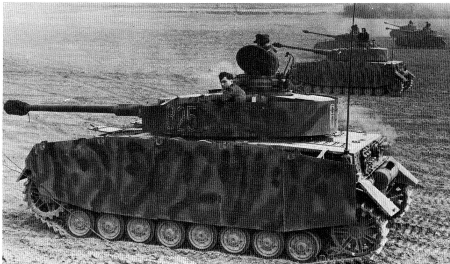
Plates 305-307. Pz Kpfw IV Ausf H. The vehicle in Plate 305 has the new type of drive sprocket but the old type of idler wheel; Plate 306 shows a late production model, with both new drive sprocket and idler wheel. Plate 307 (below): on manoeuvres in France in 1944.
