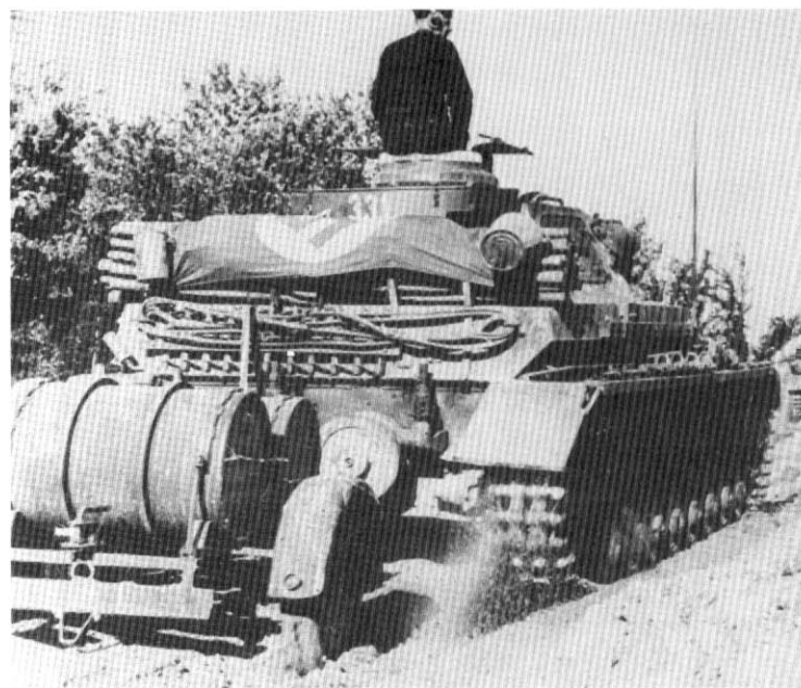
Plate 313. Tauchpanzer IV towing a fuel trailer, somewhere on the Russian Front in 1941.
