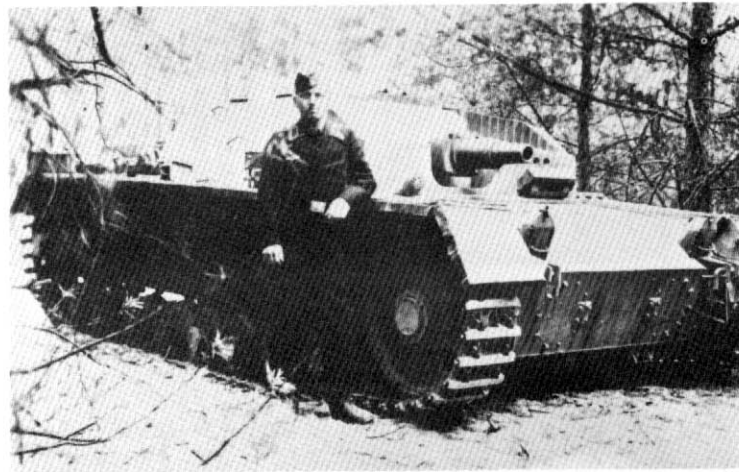
Plates 244-245. StuG III Ausf A (showing the Pz Kpfw III Ausf F suspension). Plate 246. One of the prototype (0-series) vehicles.
