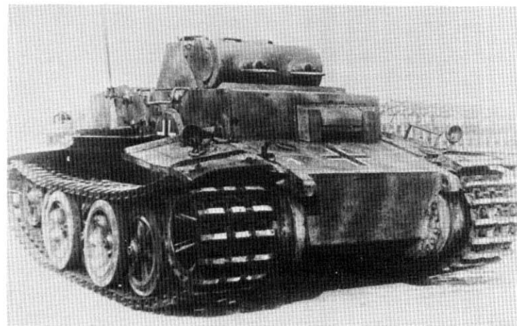
Plates 64-66. Pz Kpfw I Ausf F: Plate 65 shows the 5 periscopes in the turret roof.
