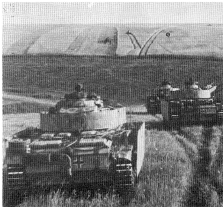
Plates 206-207. Pz Kpff III Ausf M. Note the modified exhaust valve for deep wading and the absence of both the hull escape hatch and the loader's vision port in the turret side. Right: vehicles equipped with Schürzen (armour skirts) on the Russian Front.
