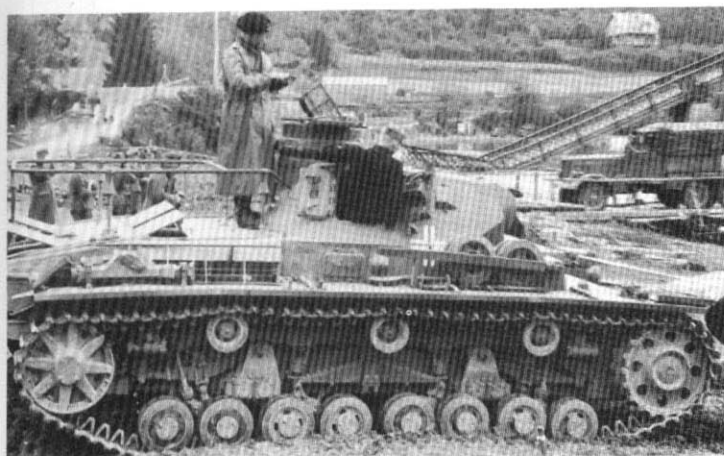
Plates 219-220. Pz Bef Wg III Ausf D 1 , showing the large frame antenna and the dummy 3.7cm gun.
