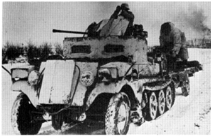
Plates 657-658. Sd Kfz 10/5; right, with armoured cab and 2cm FlaK38.
