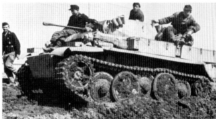
Plates 97-98. Pz Kpfw II Ausf L: Plate 97 shows the vehicle in service on the Russian Front. (Note the additional armour on the nose plate.)
