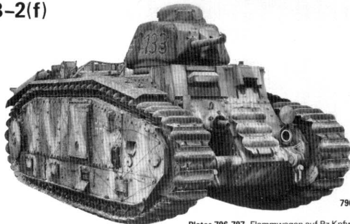
Plates 796-797. Flammwagen auf Pz Kpfw B-2(f). Plate 796 shows the flame-projector that replaced the 75mm gun in the front of the hull; Plate 797 shows the armoured fuel tank for the flame-projector, built on to the rear of the vehicle.
