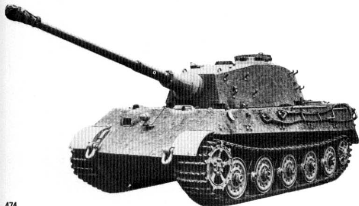
Plates 474-475. Pz Kpfw VI Ausf B with Henschel turret. Plate 476. Tiger II with wide battle tracks and track guards. Plate 477. A line-up of Tiger II vehicles, in the first battalion to receive them. Plate 478. Pz Bef Wg mit 8.8cm KwK43 L/71.
