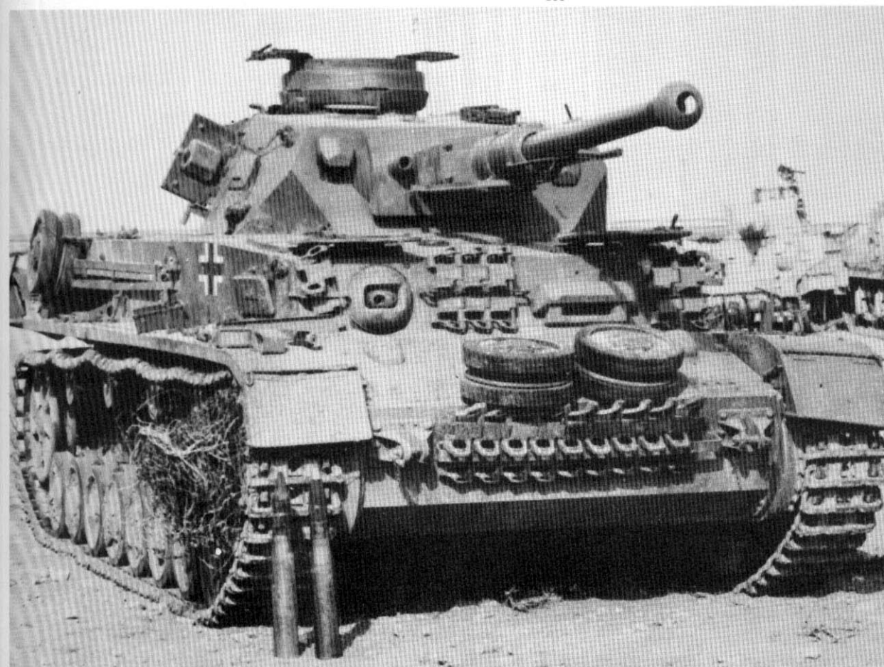
Plates 299-301. Pz Kpfw IV Ausf F 2 . The tank in Plate 300 has been captured in the Western Desert (where the model was known to the British as the 'Mk IV Special'). Fitted to the gun barrel is an aerial deflector similar to that used on the short 7.5cm gun. In Plate 301, the KwK40 gun has been fitted with the early single-baffle, globular muzzle-brake.
