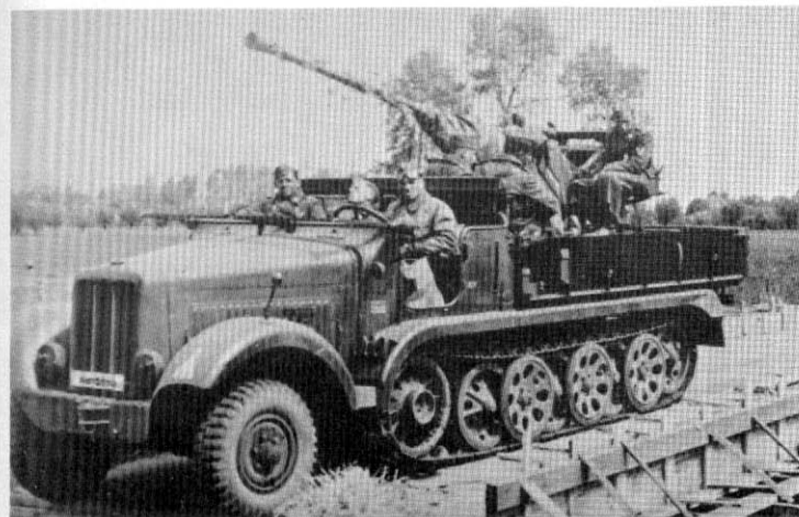
Plates 666-667. 3.7cm FlaK36 auf Fgst Zgkw 5t; right, with gun shield, and lowered sides to permit full traverse of the gun.
