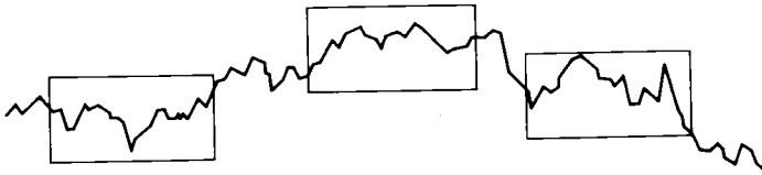
(a) A Series Showing Nonstationarity in Level such as can be Represented by the Model \phi(B)\nabla z_t = \theta(B)a_t
