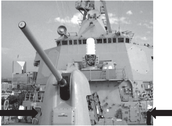
FIGURE 12.8 Spy-1D phased-array radar antennas (two of four shown). Source: After Global Security.org, 2006.
