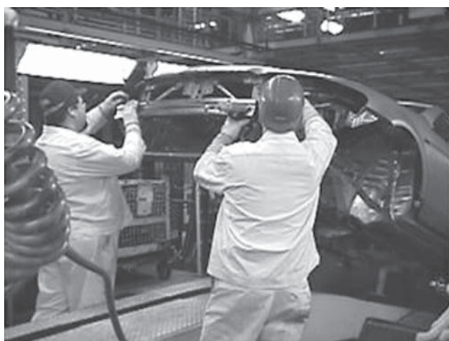
FIGURE 13.5 Installing a bumper beam on the vehicle.
