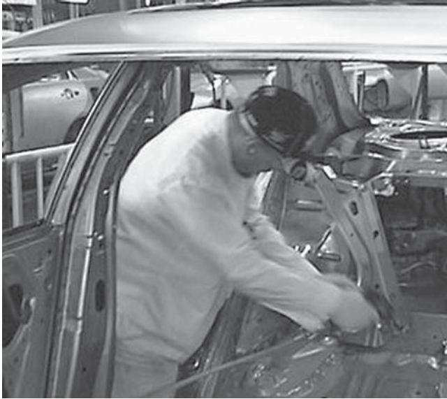
FIGURE 13.6 Attaching a gusset to the vehicle's rear bulkhead.
