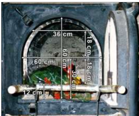
Illustration 4: Muffle door of the Topf double-muffle furnace at the Mauthausen Camp, identical to those of the double-, triple- and 8-muffle furnaces at Auschwitz. © C. Mattogno
