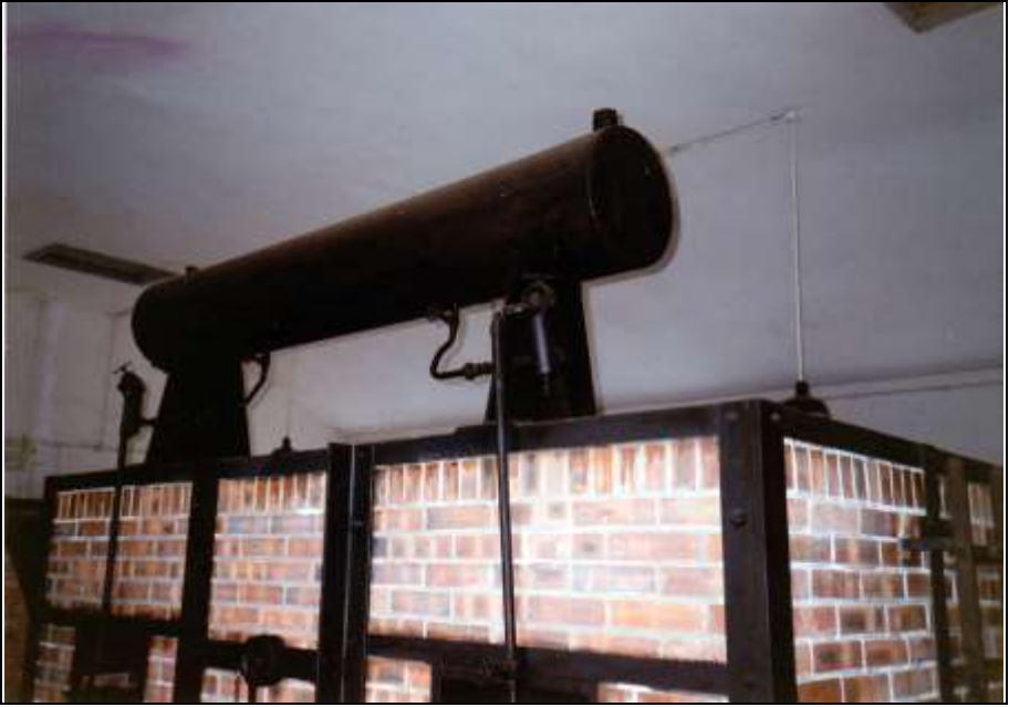
Photograph 202: TOPF coke- or naphtha-fired triple-muffle cremation furnace; naphtha tank, rear view.
