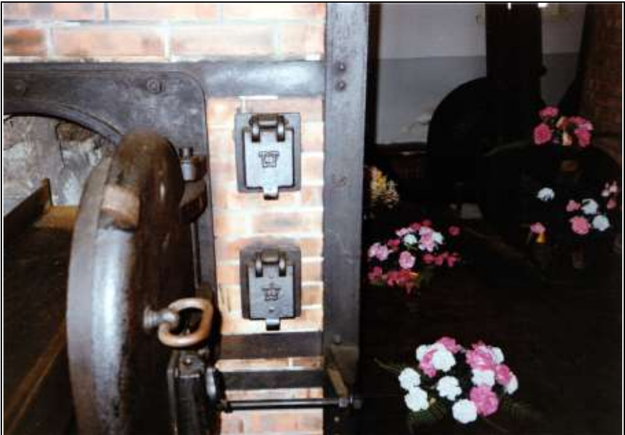
Photograph 148: TOPF coke- or naphtha-fired triple-muffle cremation furnace. Right-hand muffle. Doors closing the combustion-air channels of the muffle (top) and of the ash chamber (bottom).
