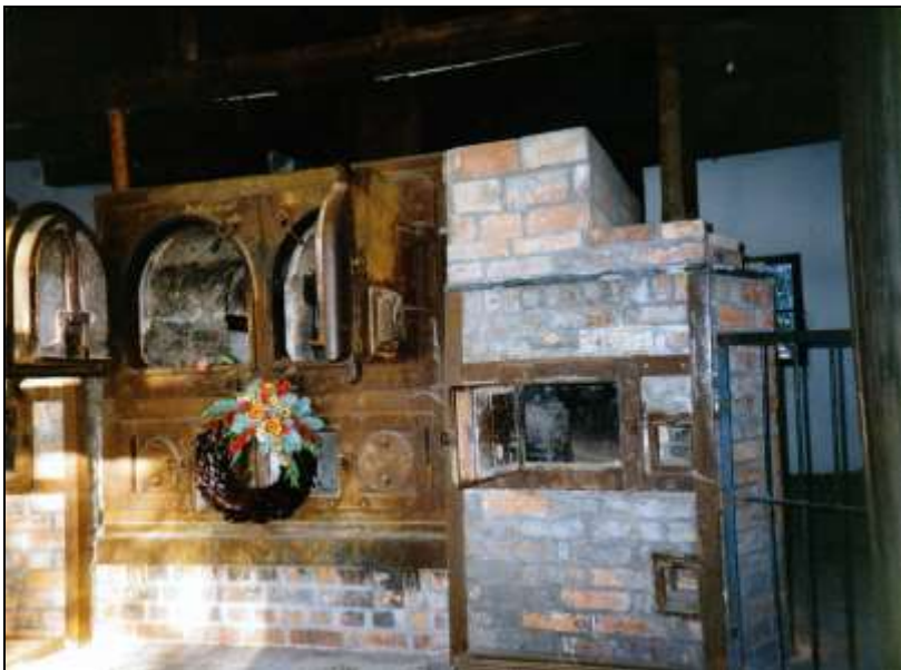
Photograph 38: Original furnace body with right-hand masonry gasifier.
