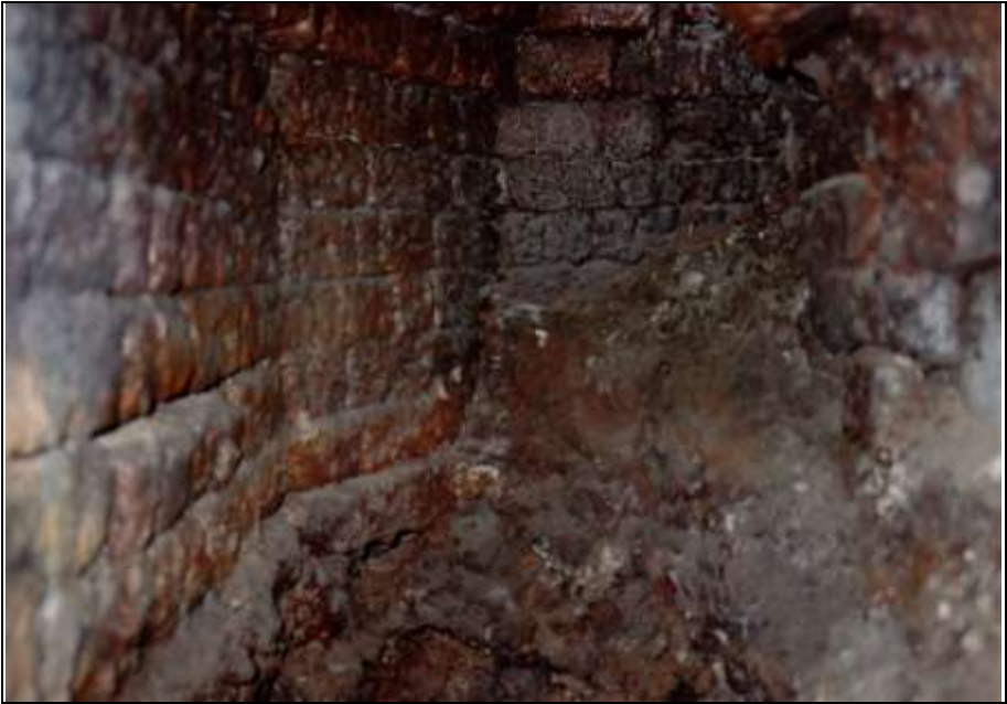
Photograph 315: Inside of the gasifier of the TOPF Furnace at Gusen Concentration Camp. The refractory lining shows extensive fusion.
