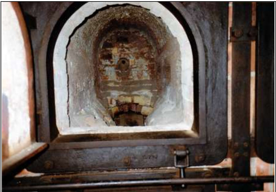
Photograph 130: same location as above, interior of the left-hand muffle of the TOPF coke- and naphtha-fired triple-muffle cremation furnace.
