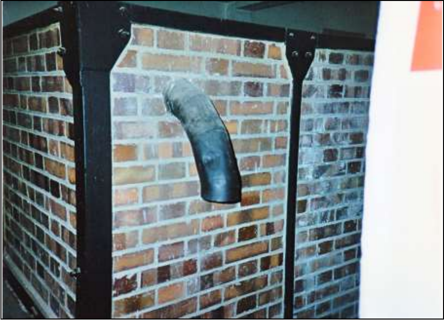
Photograph 76: Air pipe originally connected to a blower.
