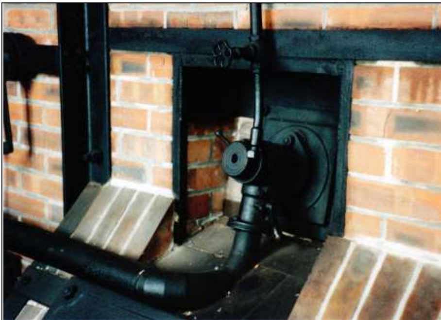
Photograph 204: as above, rear view, naphtha burner of the left-hand muffle; connected to the naphtha burner are from above, the tube feeding oil from the naphtha tank, and from below, the tube from the combustion-air blower.
