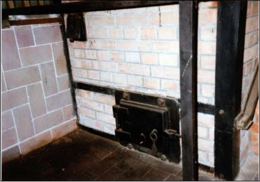
Photograph 175: Topf coke-fired triple-muffle cremation furnace. Rear view, right-hand muffle: the gasifier's ash-chamber door (bottom) and its combustion-air-channel door (top left).
