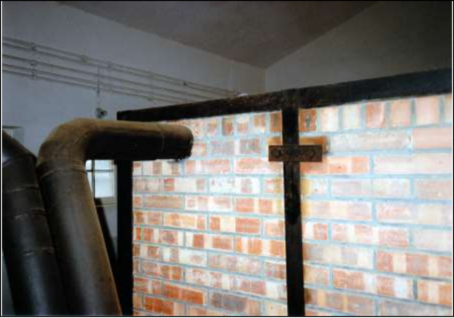
Photograph 193: Blower tube connected to the coke-fired furnace.
