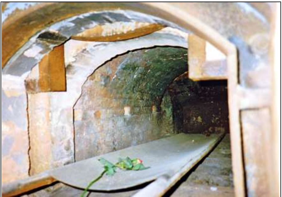
Photograph 253: Second furnace, inside the muffle; left-hand side with three openings for combustion-air supply.
