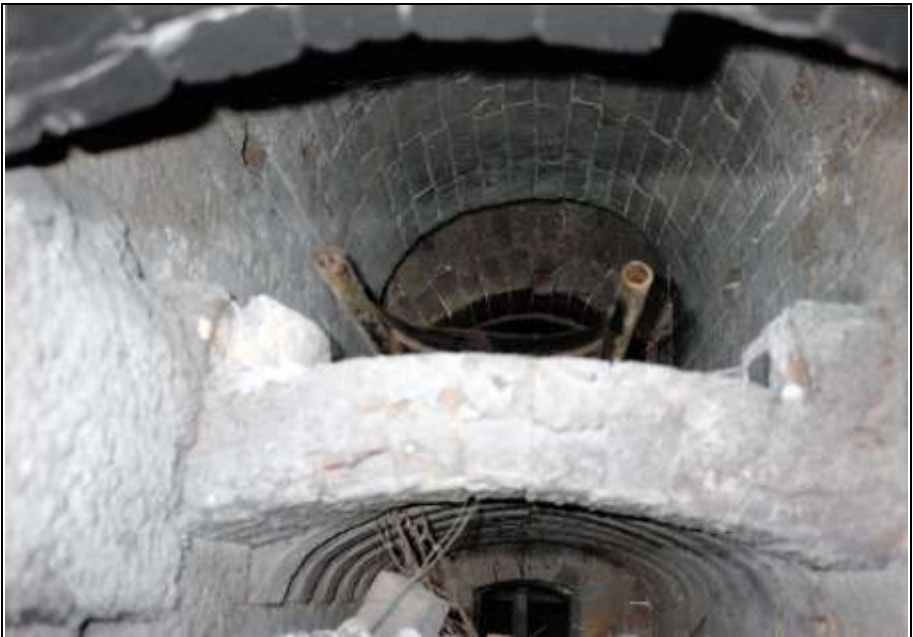
Photograph 314: as above; bottom: the ash chamber with the ash-chamber-access door in the background; above that: the muffle's fireclay grate; top: the muffle.
