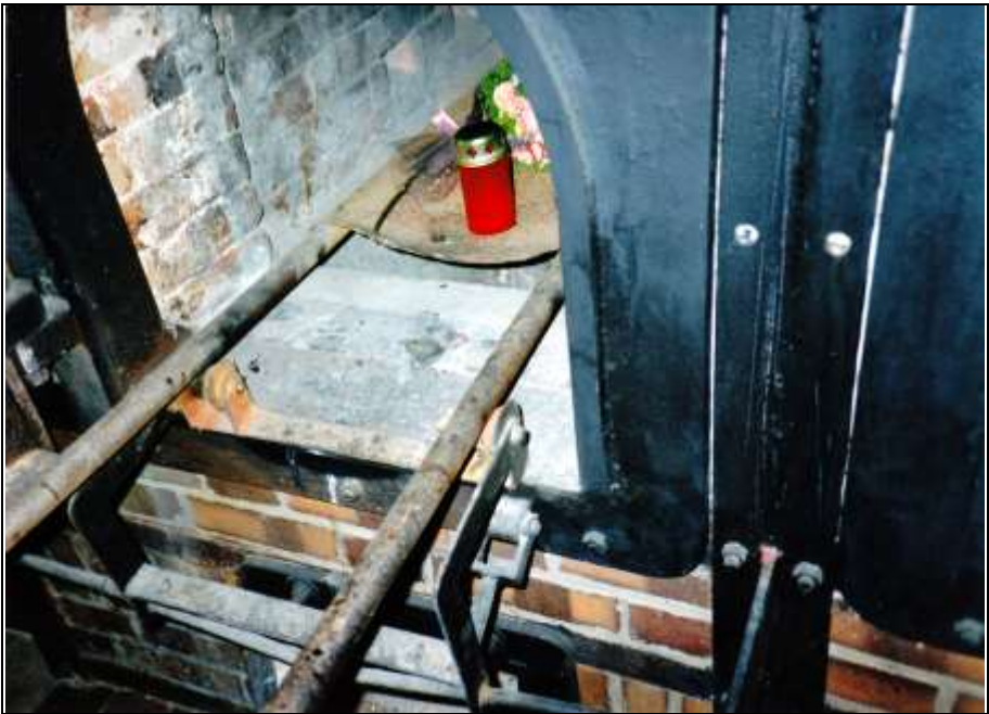
Photograph 85: as above, viewed from top: the movable roller device on which the bars of the corpse stretcher rests.
