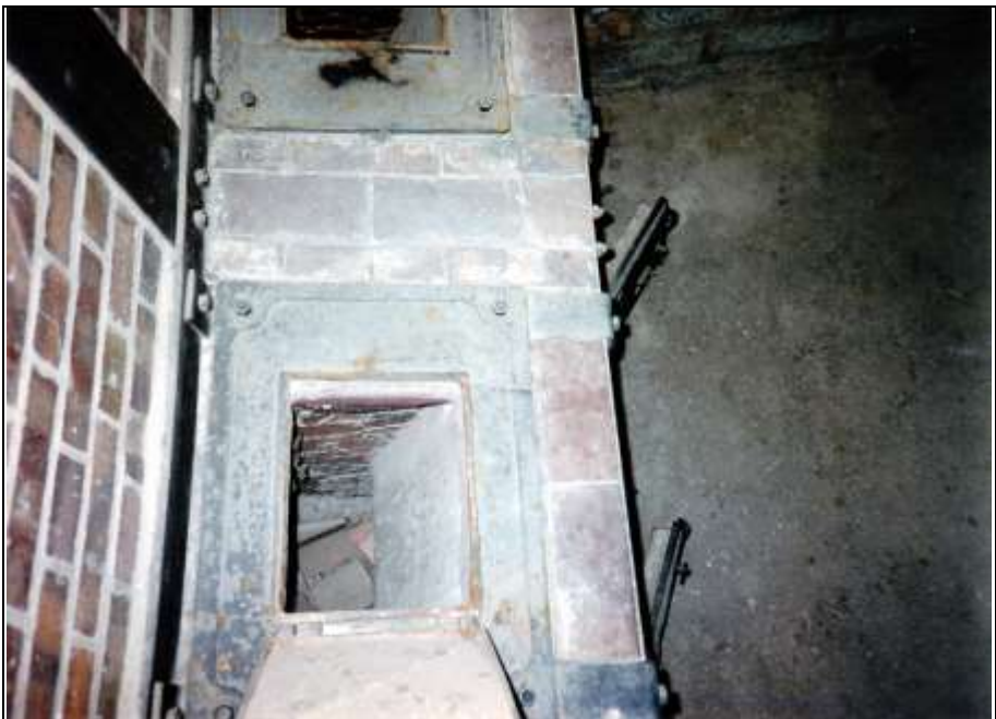
Photograph 79: as above; coke-loading door of the gasifier heating the right-hand muffle.
