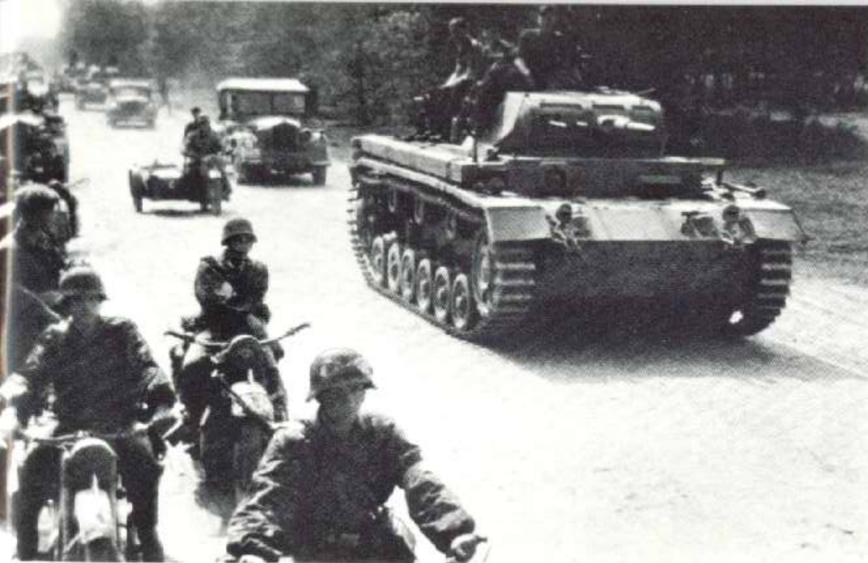
Panzerbefehlswagen III Ausf E, command vehicle, passes a resting detachment of SS motorcyclists. Although apparently armed, a dummy gun replaced the main armament in this command vehicle, leaving only the turret MG for protection.
