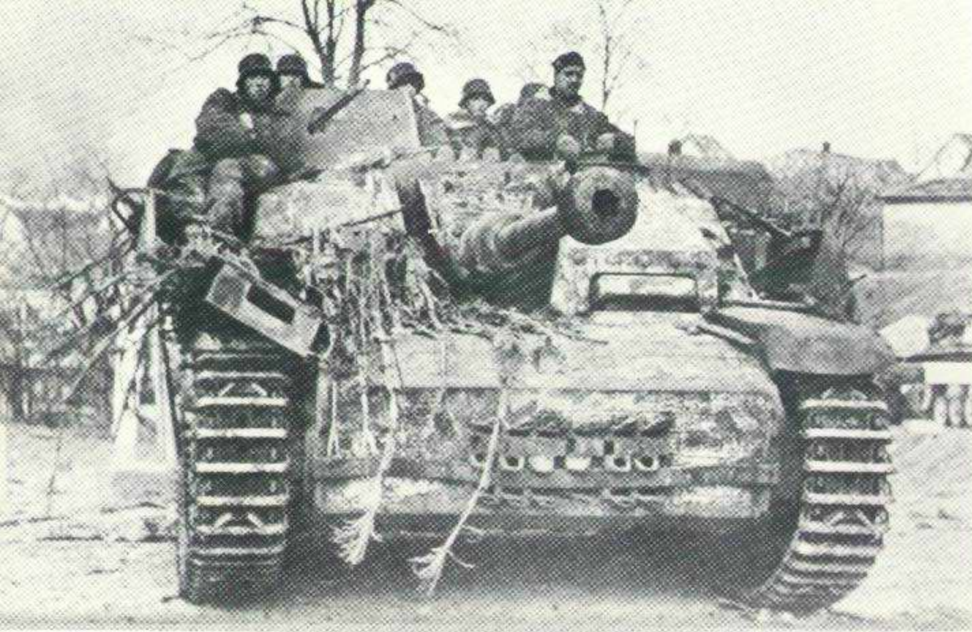
Sturm III Ausf G, late production version, featured the cast mantlet and a partially cast superstructure. By the end of 1944 Sturmgeschutzs, as a whole, had accounted for almost 20,000 destroyed enemy armored vehicles.
