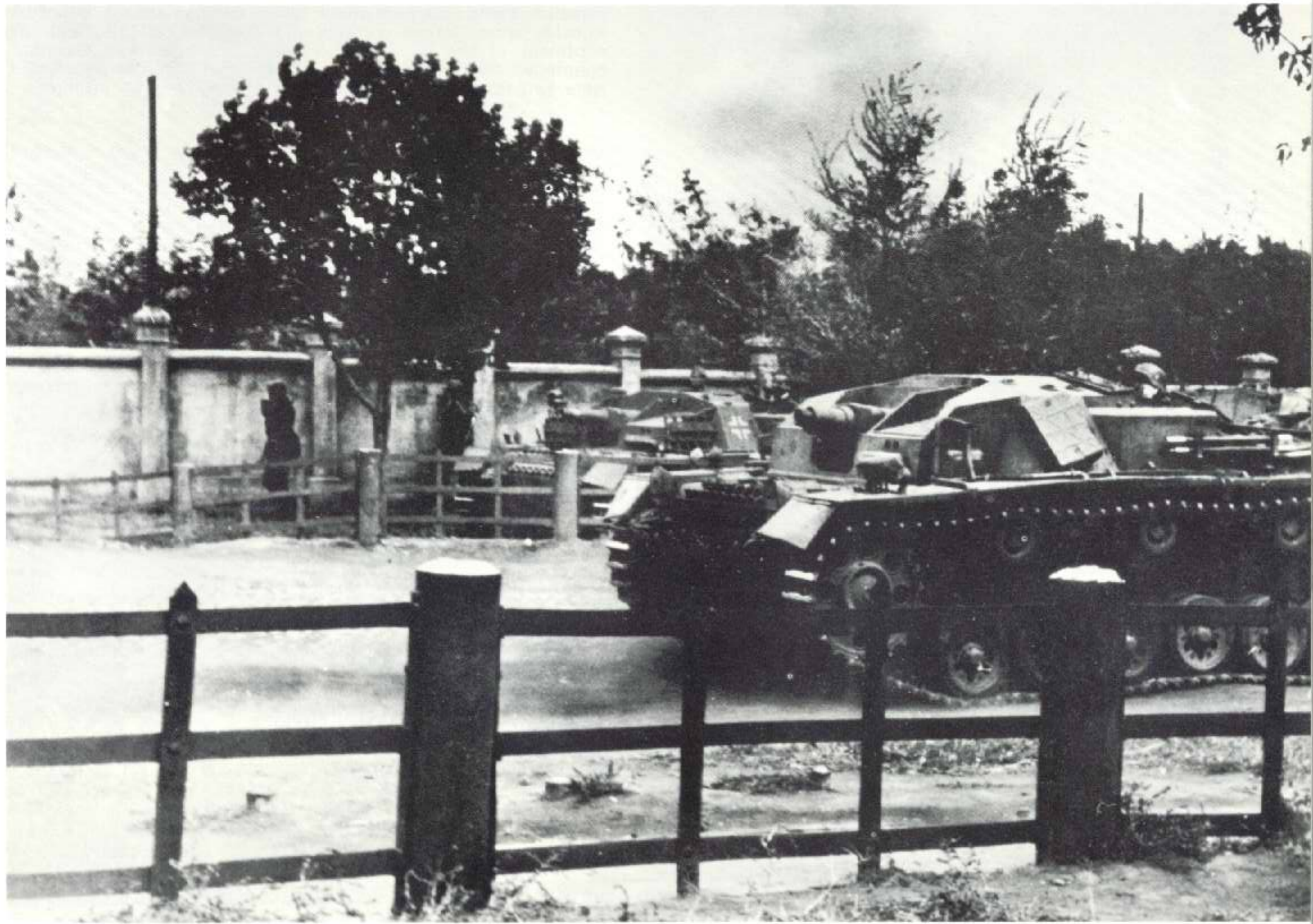
StuG III Ausf A, foreground, and StuG III Ausf C, most likely belonging to "LSSAH", June 1941. Both vehicles are armed with the short barrel 7.5cm StuK L/24 for which 44 rounds of ammunition are carried; no machine gun was carried for local defense, a feature corrected in later models. Note the gun of the vehicle in the foreground has just been fired and is in full recoil.
