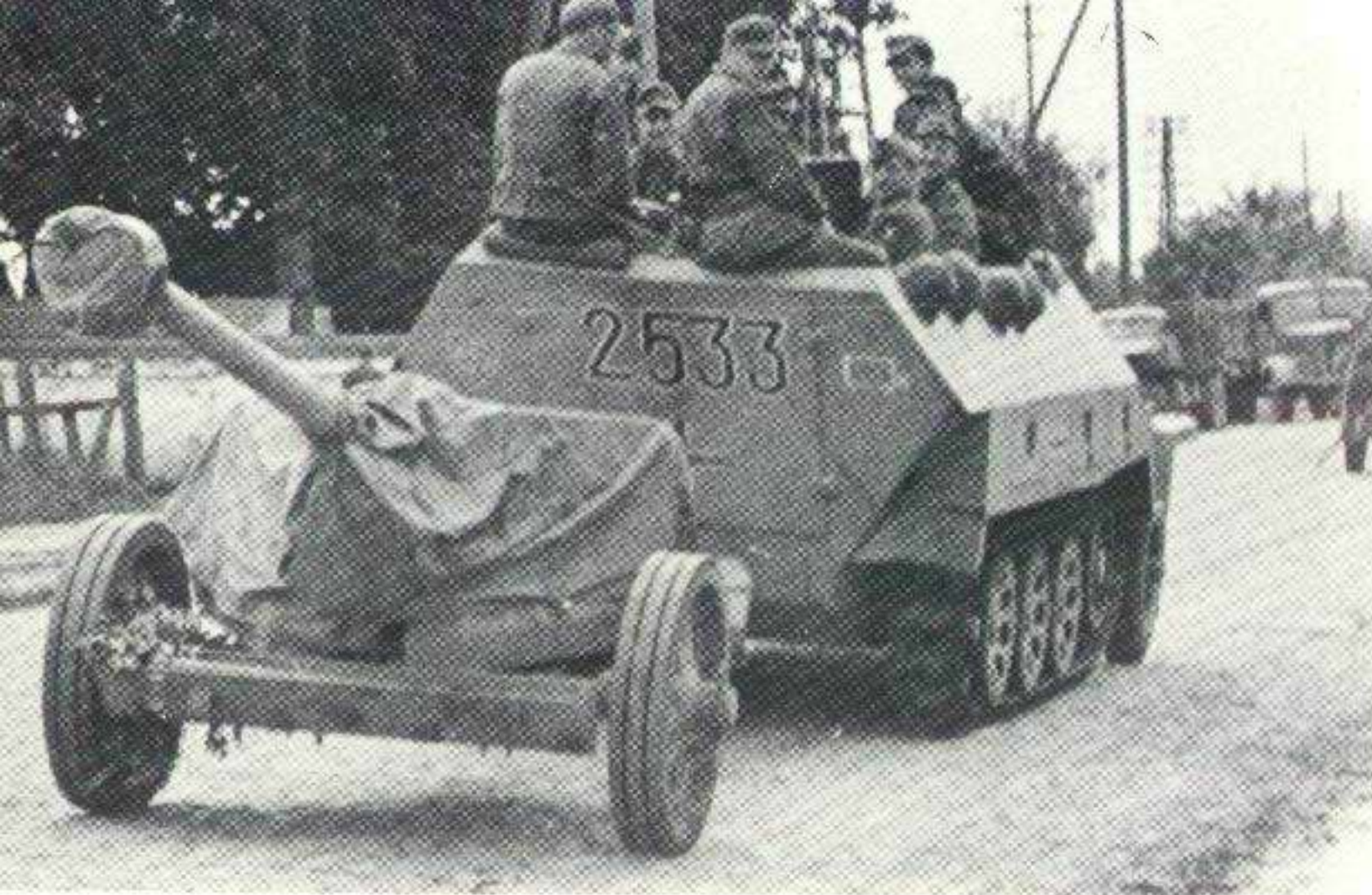
Half-track, Sd. Kfz. 251/4 Ausf D of "Wiking" division towing 7.5cm Pak.
