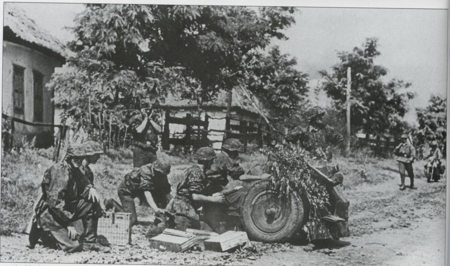
An SS gun crew mans a 7.5cm leIG 18 light gun after setting it up in position alongside a road in a Soviet village. This weapon was used on a regimental level for infantry support. Note the size of the ammunition it fires, an example of which is about to be loaded by the gunner in the center of the photo.
