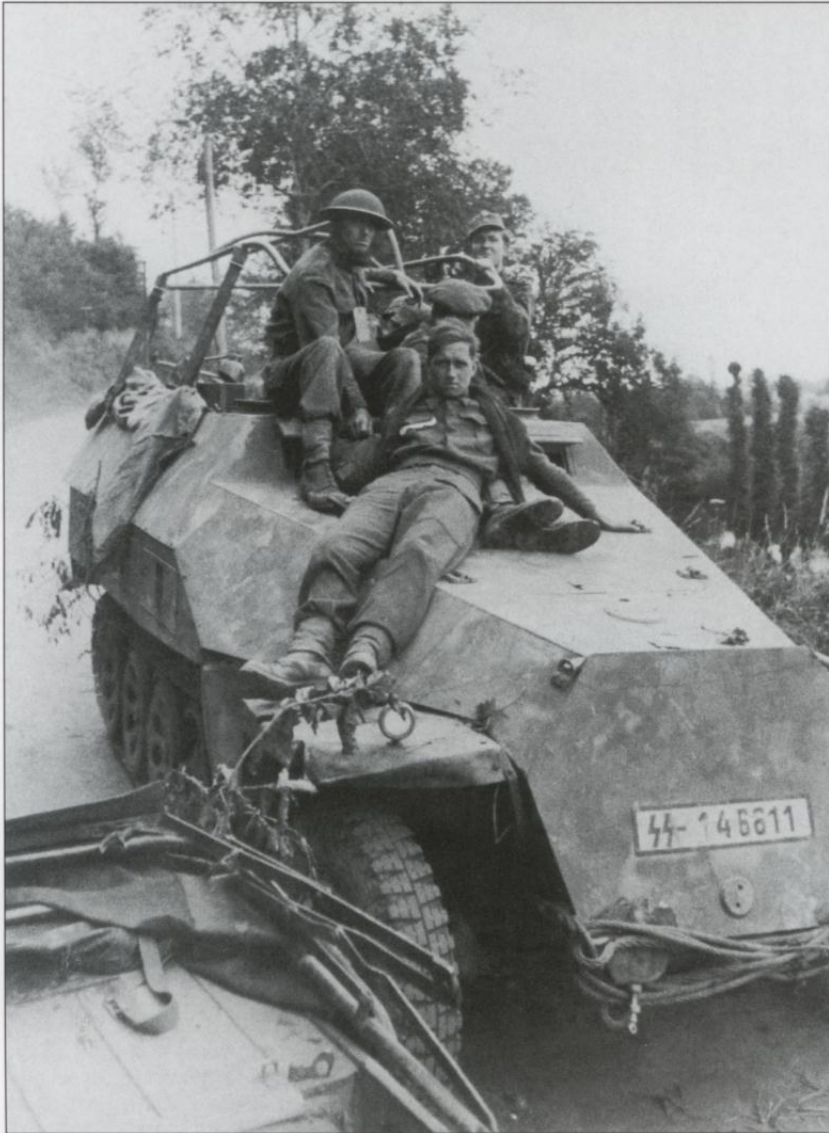
In early July 1944, an Sd.Kfz. 251 belonging to an SS reconnaissance unit is used to transport British prisoners to a command point for interrogation. The armored half-track is camouflaged with green and brown paint over a background of sand.
