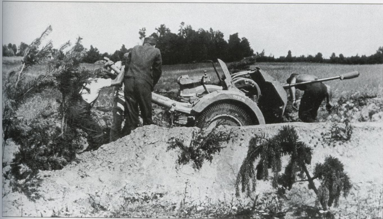
One of the most popular anti-aircraft guns used in the SS divisions was the 2cm Flak gun. It was often used against targets on land, as well — even armored ones. Here we see the crew of the Flak 38 at their battle stations preparing to put the gun into action.
