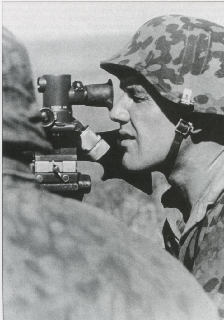
This close-up of soldiers belonging to either the 'LAH' or 'Wiking' Division shows the details of the MG34's Lafette sight, used for long-range marksmanship. Note the complex multicolor spot pattern on the camouflage material.
