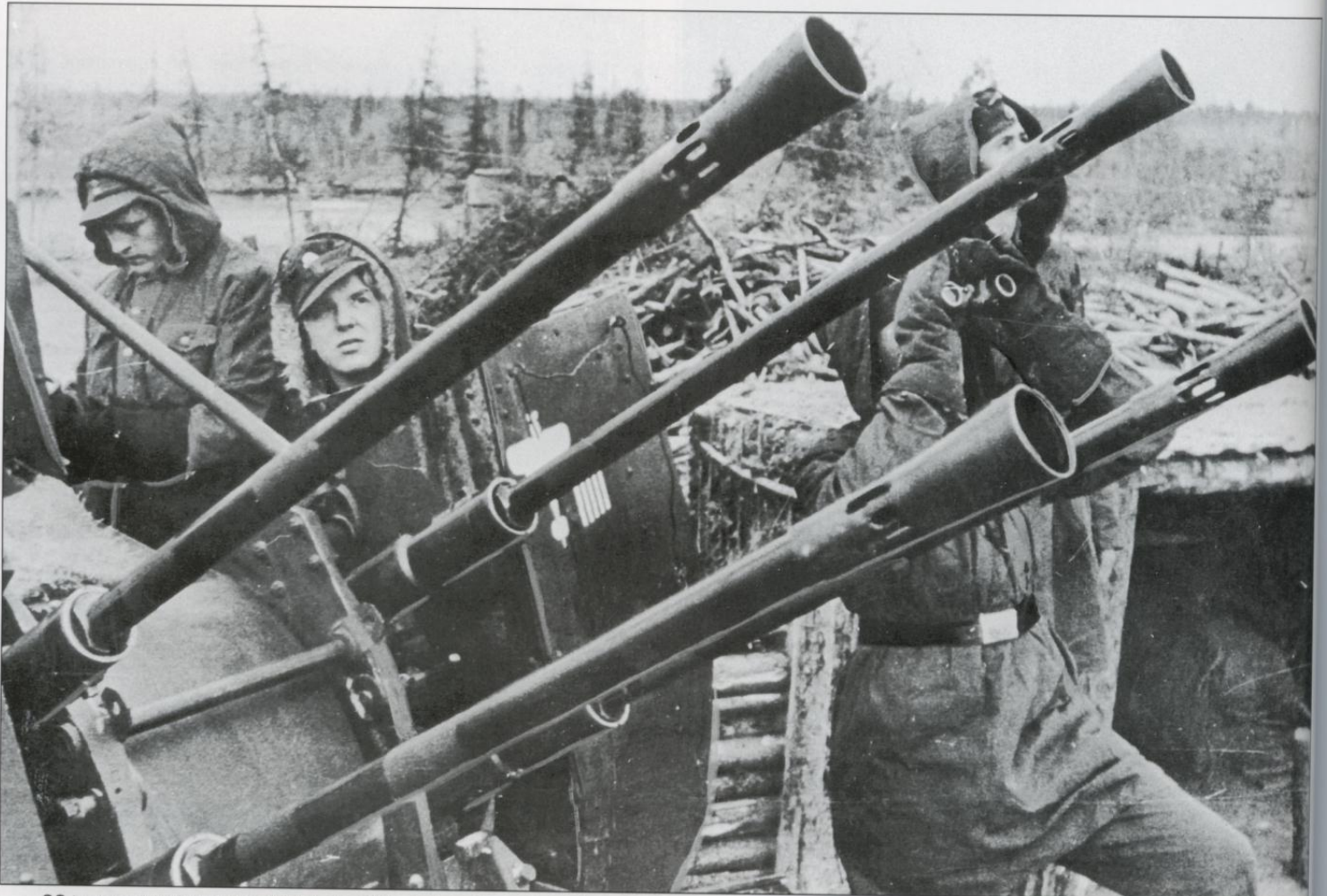
SS troops manning a 2cm Flakvierling 38 anti-aircraft gun stay alert as they search for enemy aircraft flying within range of their battery. Note the victory markings on the gun shield showing they have shot down five aircraft. The crew and the gun are camouflaged with gray, which is the best color for blending in with the landscape in the late autumn and early spring in the Soviet Union.
