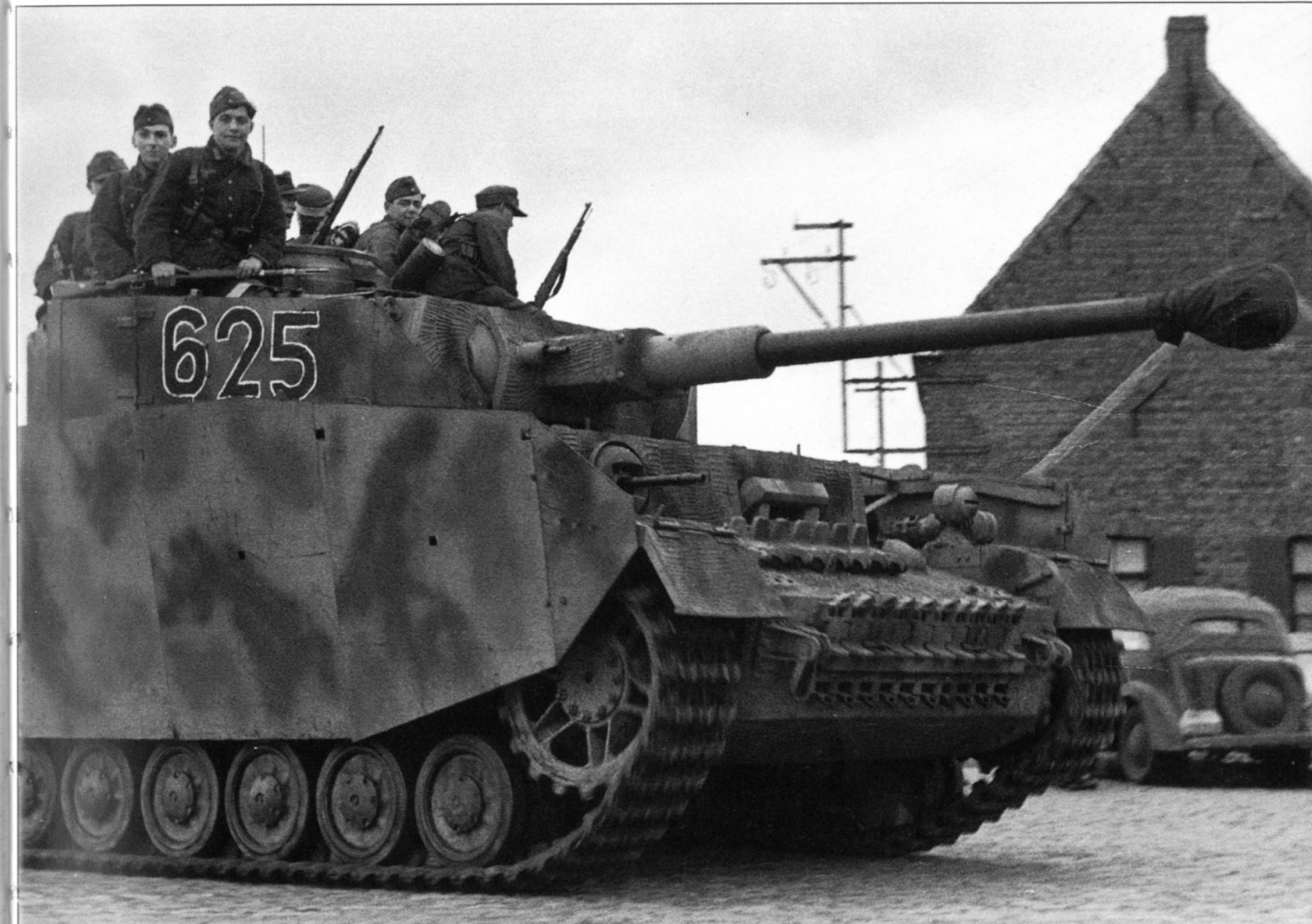
■ Below: A Hitlerjugend Panzer IV rumbles through Caen. Note the armoured "skirt" to defeat Allied antitank rockets.
