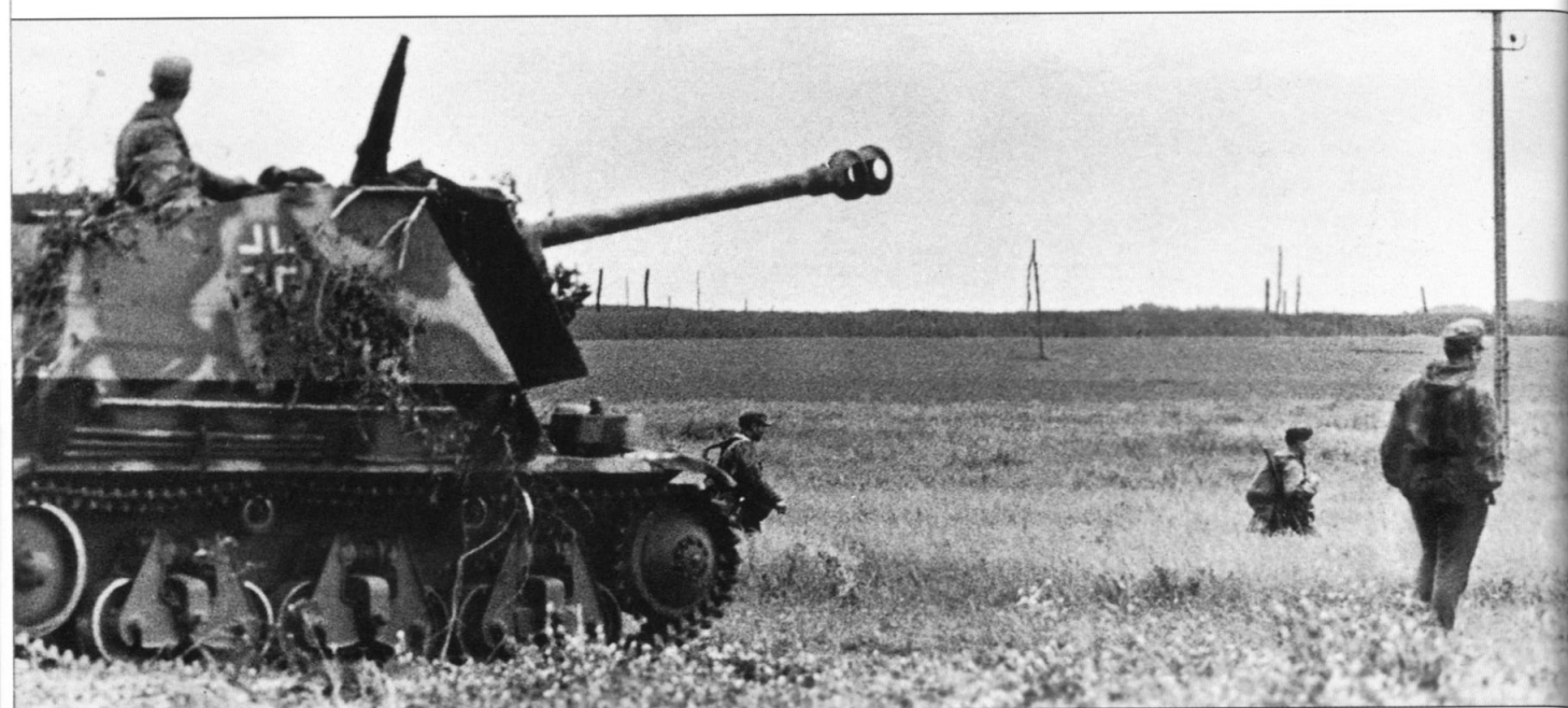
■ Above: Many German units in Normandy relied on captured vehicles, such as the H39 self-propelled 105mm howitzer based on a Hotchkiss chassis, to augment their firepower.
