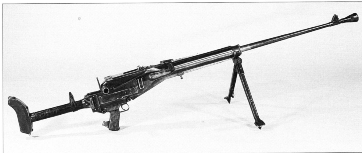
BELOW: A 7.92mm Panzerbüsche 38 anti-tank rifle. Note the bipod mount, shoulder stock and taper-bore barrel for increased muzzle velocity.
