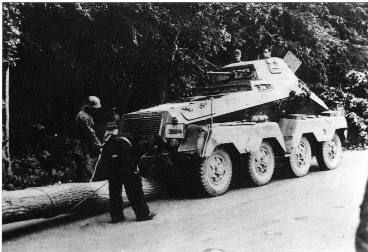
ABOVE: An SS eight-wheeled Sdkfz 231 heavy armoured car in France, May 1940. This vehicle was armed with a 20mm gun and 7.92mm machine gun.
