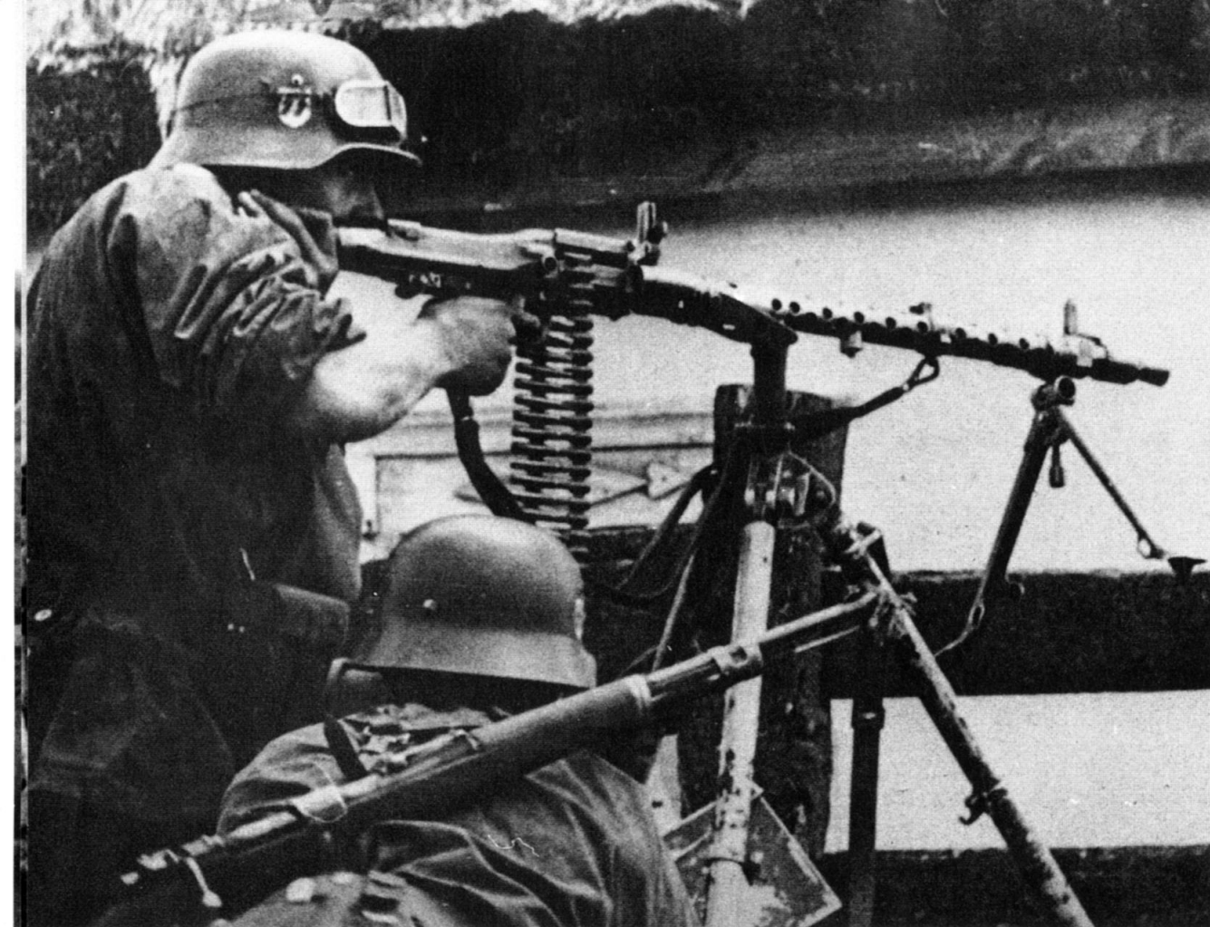
ABOVE: An excellent view of a 7.9mm MG 34 on a Dreifuss anti-aircraft tripod mounting. The ammunition feeder carries a Karabiner 89k rifle.
