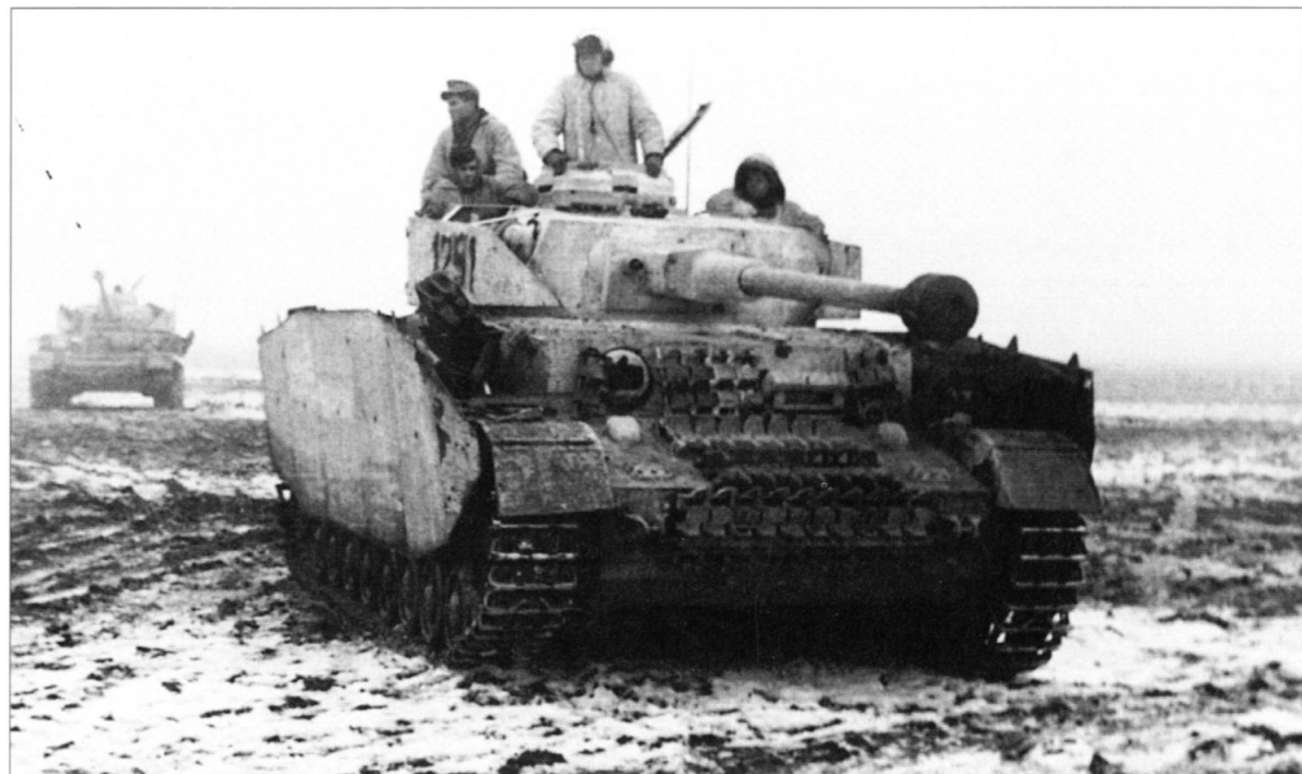
ABOVE: A Leibstandarte Panzer IV Model J tank with Schürzen aprons and Zimmerit anti-magnetic mine paste. Note the spare track sections on the hull front.
