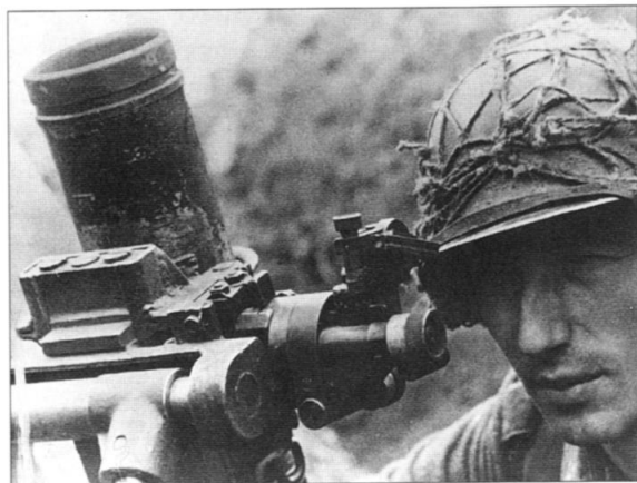
LEFT: An excellent view of a mortar operator ranging a kurzer 8cm GrW 42 . A smaller, lighter version of the 8cm GrW 34 , it was intended for airborne forces use.
