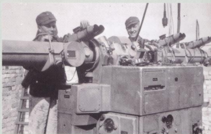
Above: Luftwaffenhelfer operating the Kommandogerät 40 (command device 40) of the battery 3./406 in the Flak Gruppe Halle-Leuna. Albrecht Riedel.
