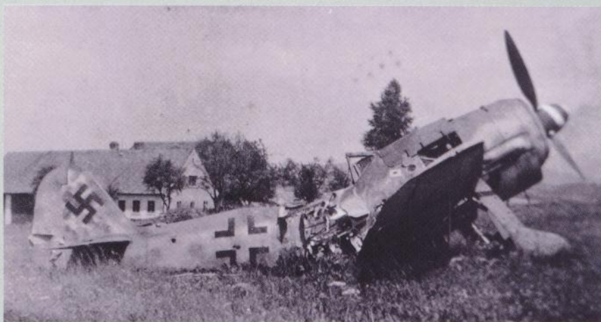
Above: Broken Eagle (I). Fw 190A-8 'Yellow 9', probably of Stab/JG6, rests with its back broken at Reichenberg airfield, May 1945. JaPo.
