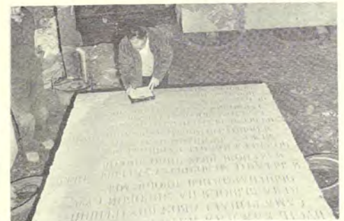
George Gaines, Chief Inspector for E.G.A.'s Certified Memorials Program, closely examined each of the units as it was completed to guarantee that each piece was free of defects and met specifications. The special E.G.A. seal certifying inspection was sandblown on each unit.
