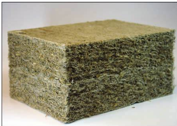
FIGURE 16.7 Hemp fiber batt insulation. Photo by Christian Gahle, nova-Institut GmbH (CC BY 3.0).
