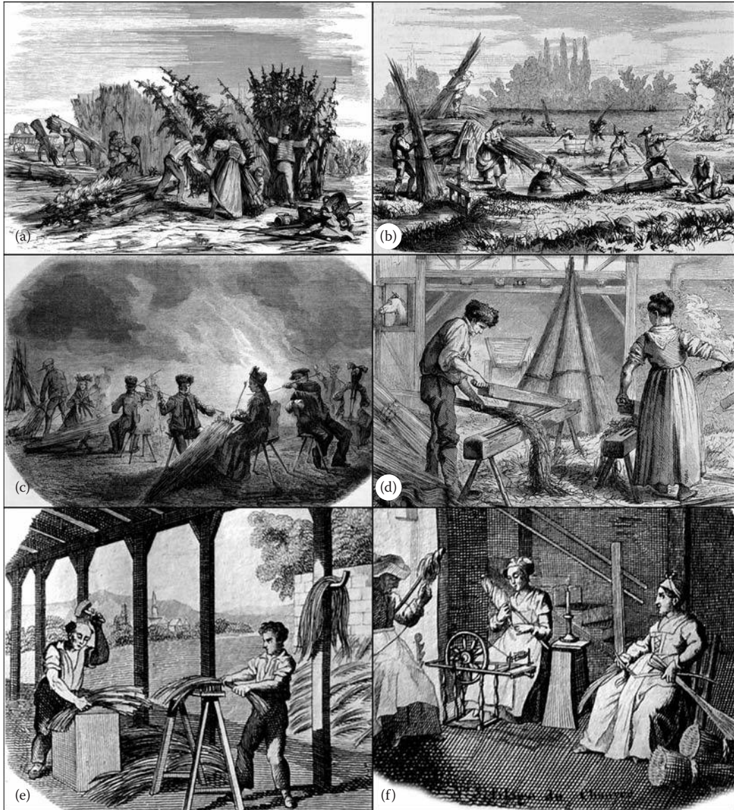
FIGURE 7.5 Traditional nineteenth century European hemp extraction and processing technologies. (a) Cutting down plants at base. (b) “Water retting,” the process of immersing stems for a week or more, so decay microorganisms loosen attachment of fiber to other tissues. (c) An alternative to retting: hand-stripping the fiber-bearing “bark.” (d) Using a “hand break” to crudely separate fiber from retted stems. (e) Left: Beating dried hemp stalks with a hand tool to crudely separate fiber from retted stems. Right: Hackling (drawing partially cleaned hemp bark fiber through a bed of nails to clean off remaining undesired tissues). (f) Spinning fiber into thread. (a–d) From Lallemand, M.G., Levy, M. 1860. L'illustration Journal Universel 926, 1860. (e and f) From Anonymous, Galerie industrielle , Eymery, Paris, France, 1822 (in French).
