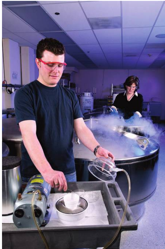
FIGURE 17.4 Ultracold cryopreservation laboratory of the Agricultural Research Service, USDA. Materials are stored long-term in “cryovats” of liquid nitrogen. (Public domain photo.)
