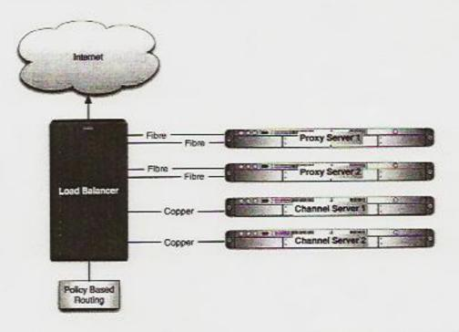
In operation, user TCP port 80 traffic was redirected using Policy Based Routing through a Load Balancer, configured to use TCS (transparent cache switching). This redirected TCP port 80 traffic to the two real proxy-servers.
