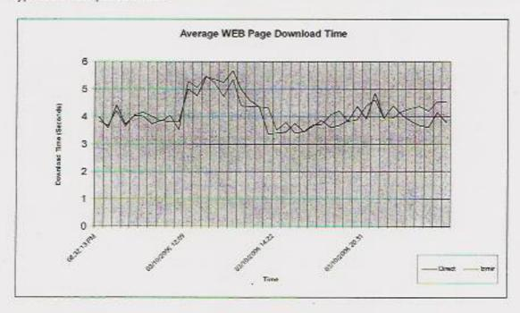
As indicated, there is very little perceptible difference between the direct and PageSense connections, all pages being delivered in between 3-6 seconds during both peak and off-peak periods in both cases.
