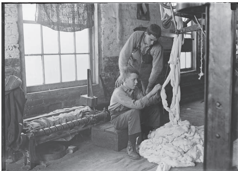
FIGURE 2. This scene from Tennessee textile mill depicts the typical case of young laborers training each other on the job. The boys are working at a warping machine. Lewis Hine, 1910. Library of Congress, Prints & Photographs Division, National Child Labor Committee Collection, LC-DIG-nclc-05391.
