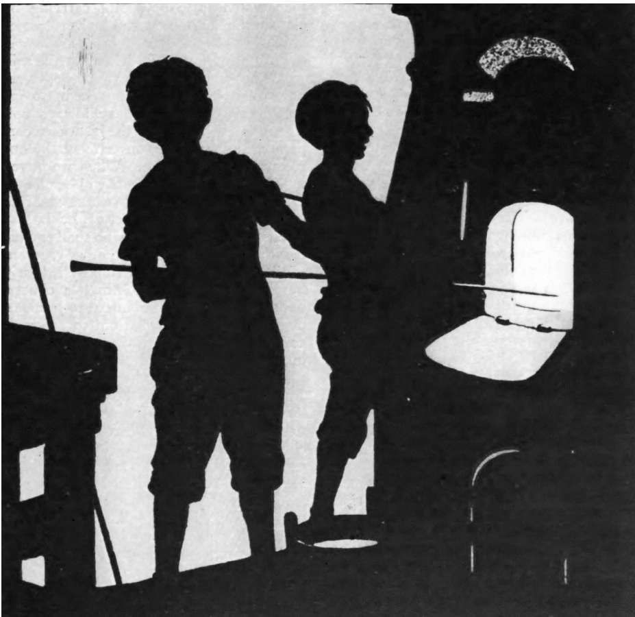
Woodcut showing boys working at the red-hot furnace of a bottle factory, 1906. The mold-holding boys heated the glass to a molten state and carried it to the adult glassblower. Once the bottle was shaped, the carrying-off boy took it to the finisher and from the finisher to the cooling kiln. The cleaning-up boy cleaned the ends of the blowpipe between uses. Image from Cosmopolitan Magazine , September 1906.
