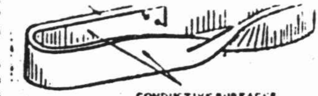
Moebius loop resistor has only one continuous conducting surface. Dielectric material separates opposing surfaces of the conductor. Leads are exactly opposite.
