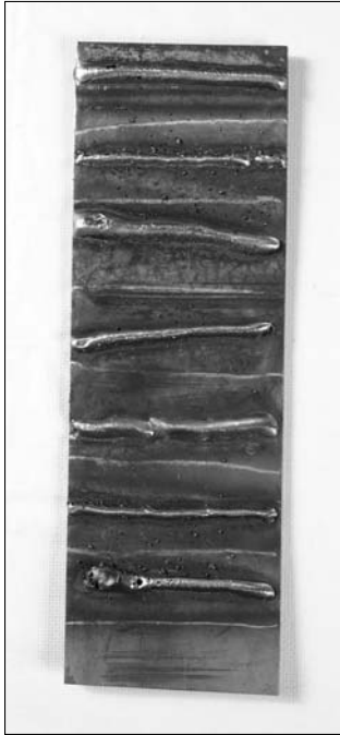
Figure 10-2: Examples of mig weld beads, from top to bottom: Good, too fast, too slow, voltage too low, voltage too high, WFS too low, WFS too high
