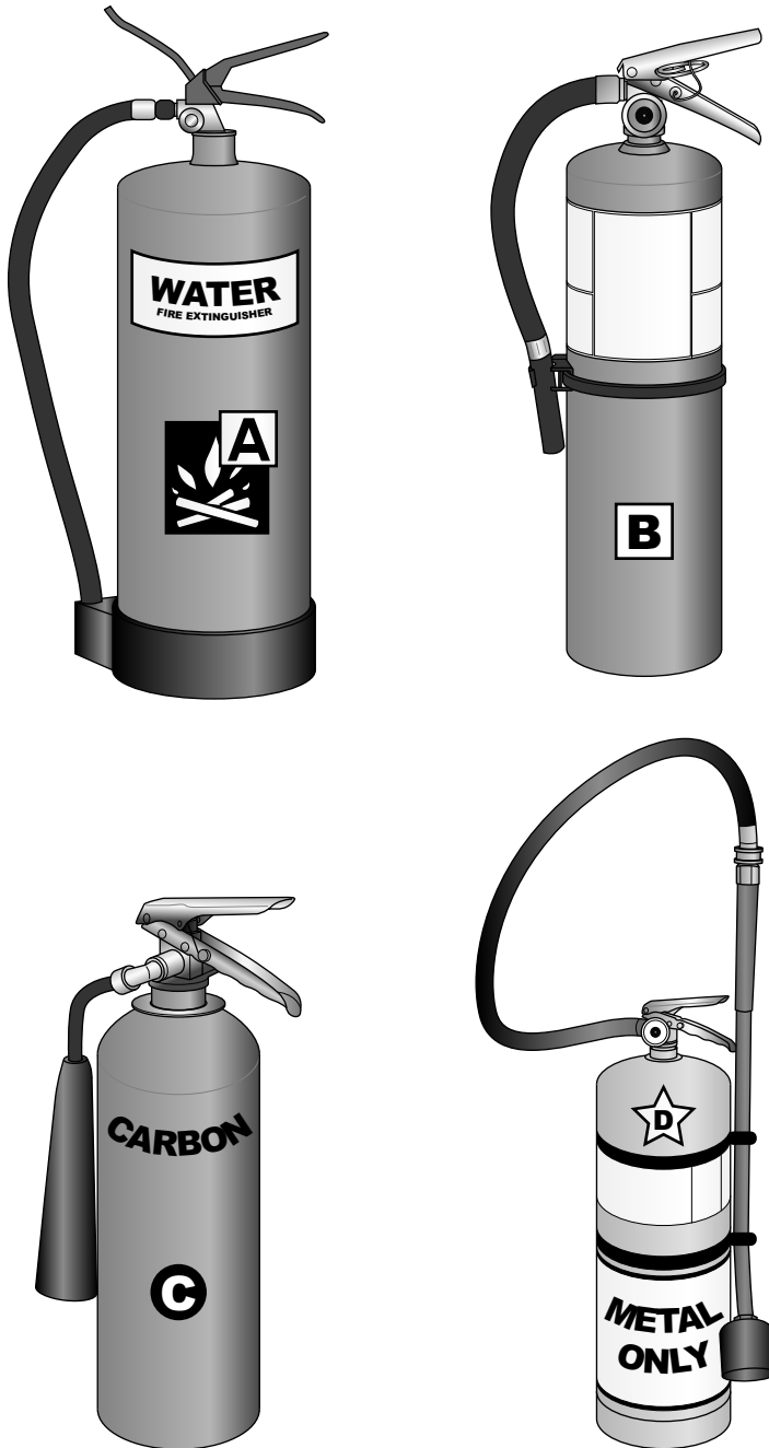
Figure 3-2: Four classes of fire extin- guishers.
