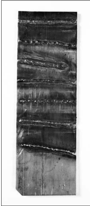
Figure 6-3: Examples of seven stick welds of varying quality.
