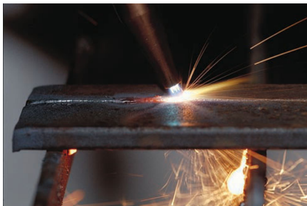
Figure 6.43 Good cut showing a steady stream of sparks flying out from the bottom of the cut
