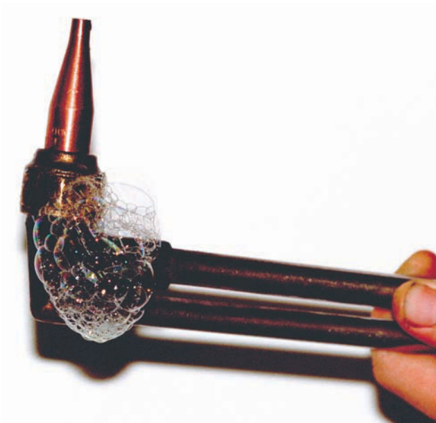
Figure 6.15 Checking a cutting tip for leaks
