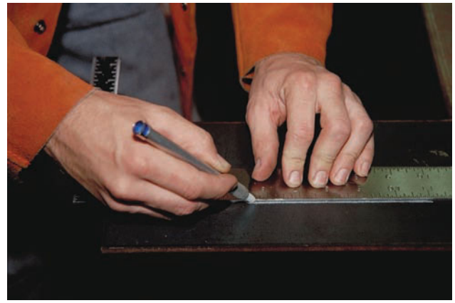
Figure 4.20B Using a straight edge to make a line
