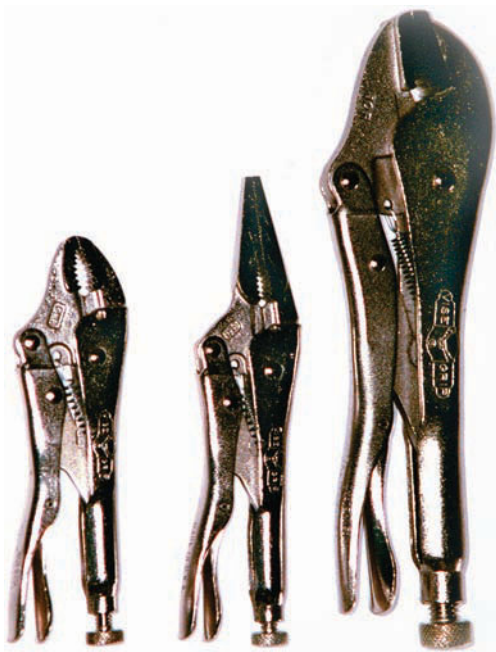
Figure 4.33 Three common types of locking jaw pliers Source: Courtesy of Larry Jeffus
