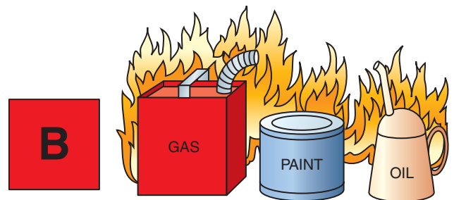
Figure 2.29 Type B fire extinguisher symbol
