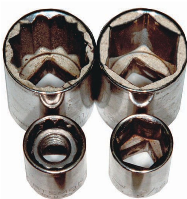
Figure 2.38 Wrench slippage The fewer the points, the less likely the wrench is to slip Source: Courtesy of Larry Jeffus
