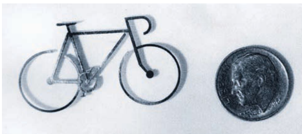
Figure 8.8 Detailed small part not much larger than a dime made with a laser
