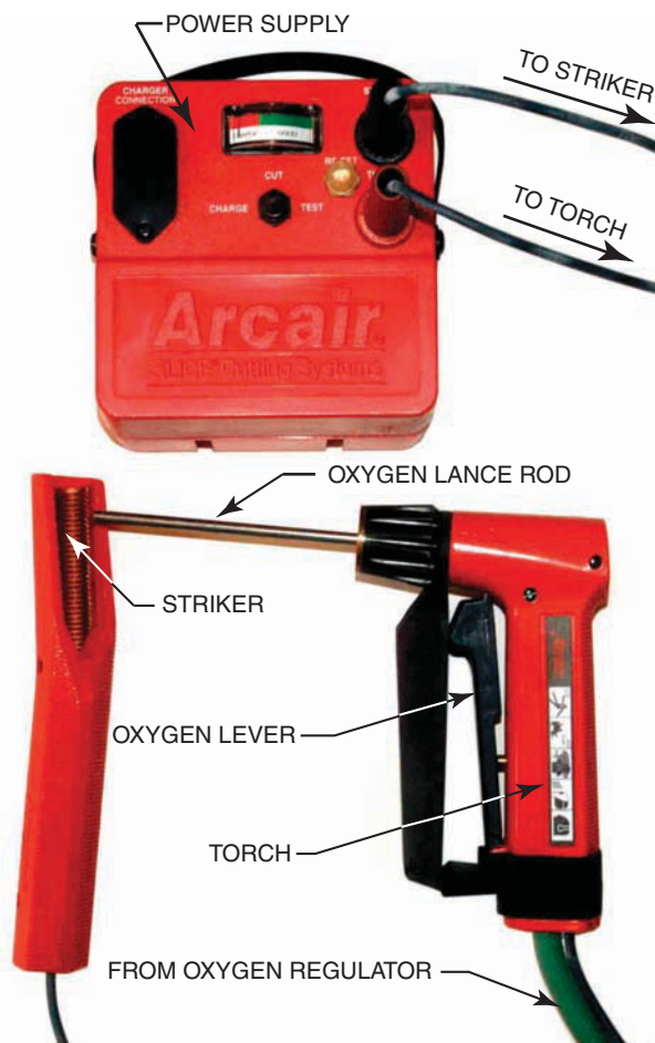
Figure 8.26 Oxygen lance cutting
