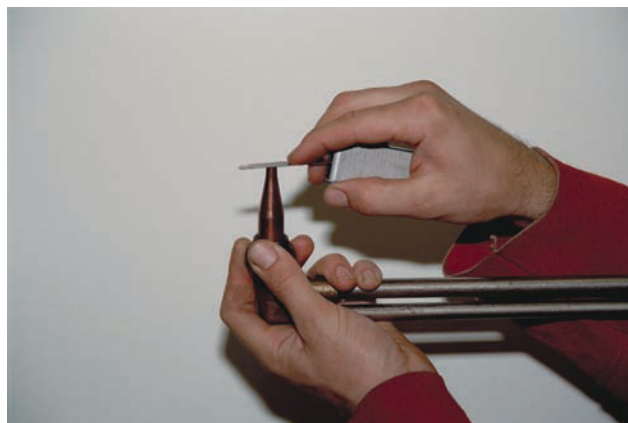
Figure 6.19 Filing the end of the tip flat
