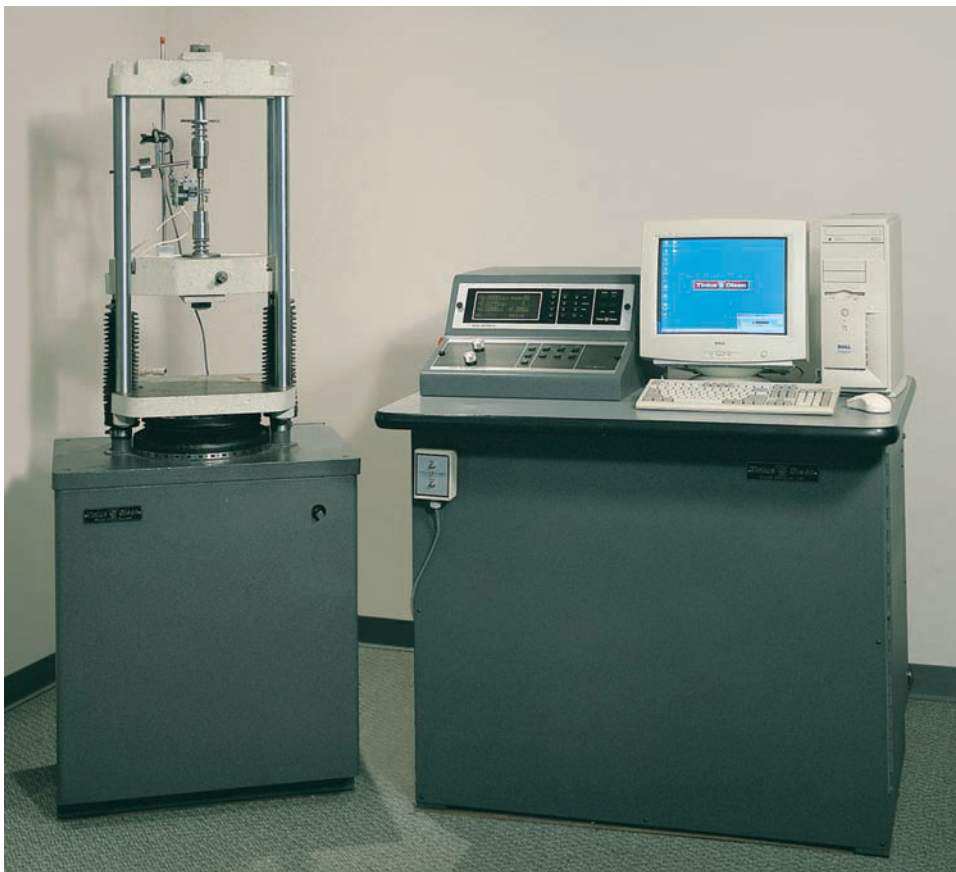
Figure 9.21 Typical tensile tester used for measuring the strength of welds (60,000-lb universal testing machines) Source: Courtesy of Tinius Olsen Testing Machine Co., Inc.
