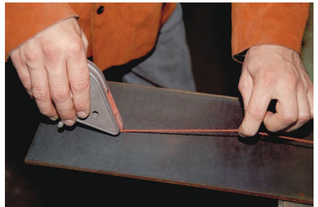
Figure 4.6A Chalk lines Pull the chalk line tight and then snap it Source: Courtesy of Larry Jeffus
