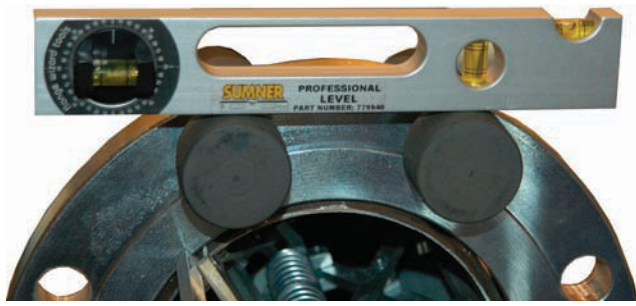
Figure 4.35A Pipe alignment clamps and level
