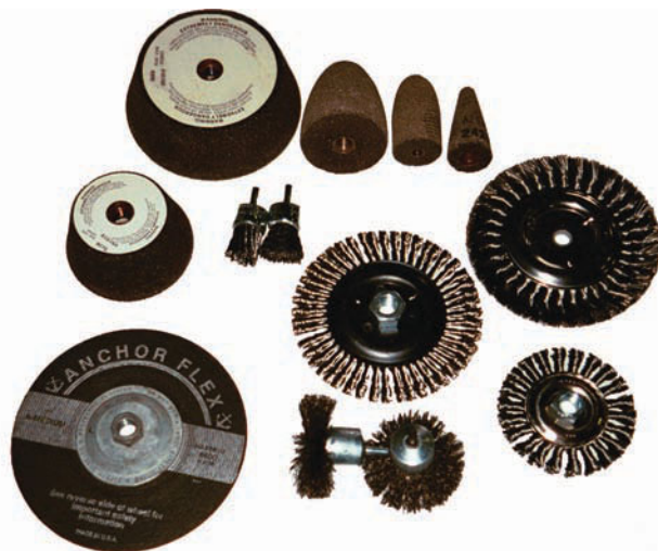
Figure 4.40 Wire brushes and grinding stones used to clean up welds
