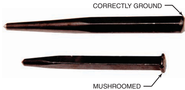
Figure 2.39 Punches and chisels
