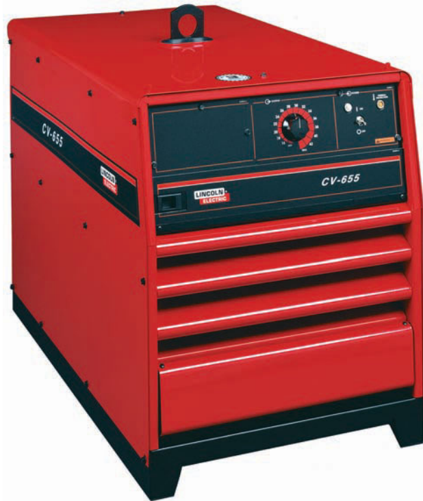
Figure 1.29 Two power supplies for multipurpose GMAW applications
