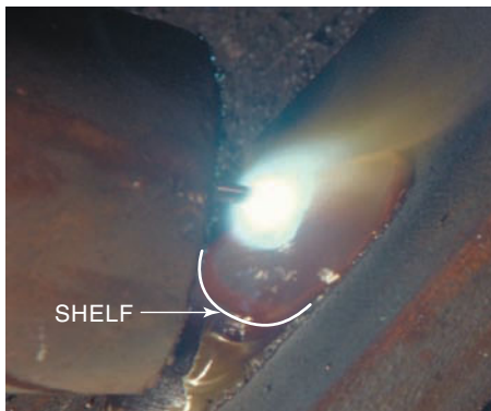
Figure 2.34 Vertical up position Source: Photo courtesy of Larry Jeffus
