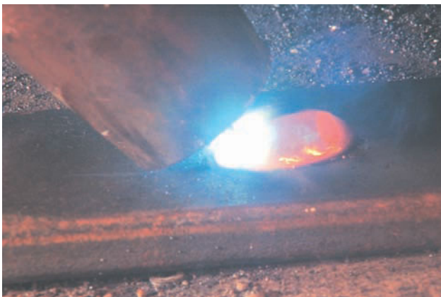
Figure 1.21 Backhand welding, or drag angle Source: Courtesy of Larry Jeffus
