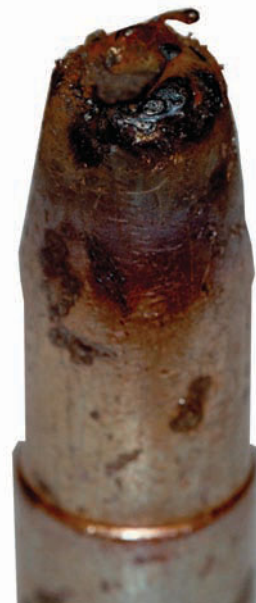
Figure 2.44 Gas nozzle damaged after shorting out against the work
