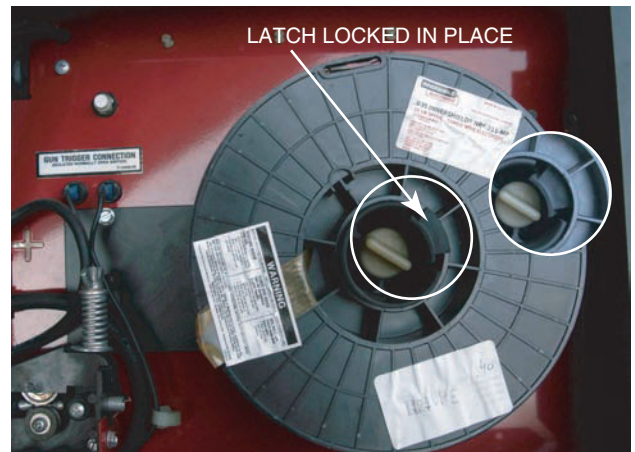
Figure 4.4 Wire reel may be secured by a center nut or locking lever Source: Courtesy of Larry Jeffus
