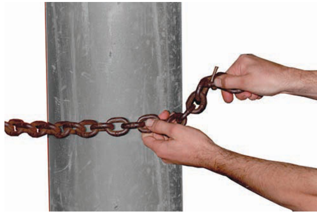
Figure 2.2 Make sure the gas cylinder is chained securely in place before removing the safety cap
