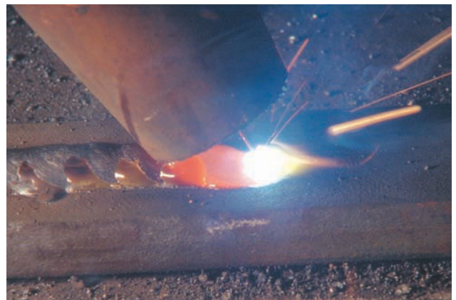
Figure 1.22 Forehand welding, or push angle Source: Courtesy of Larry Jeffus
