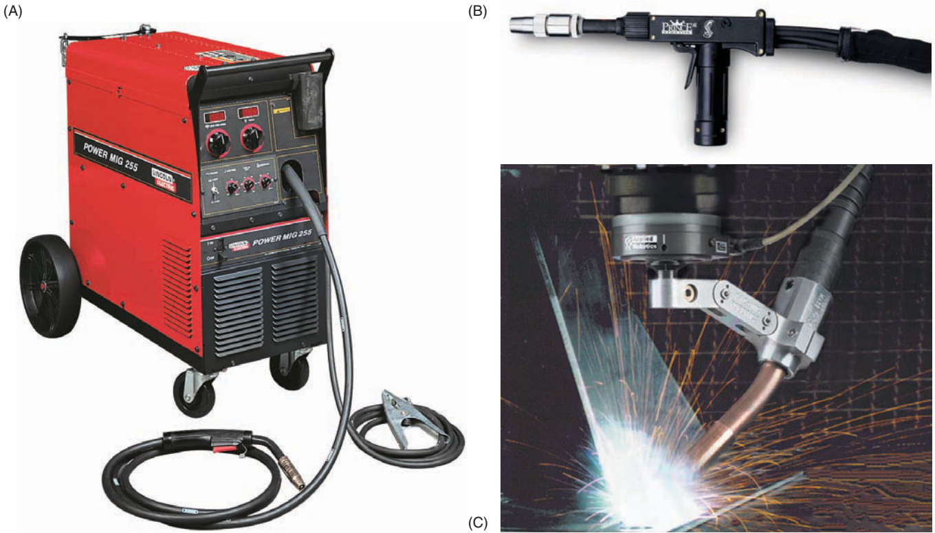
Figure 1.2 GMAW equipment (A) Semiautomatic GMA welding setup. (B) Machine GMA welding gun with a friction drive, which provides both uniform nozzle-to-work distance and travel speed. (C) Automatic GMA welding. Source: Courtesy of Lincoln Electric Company
