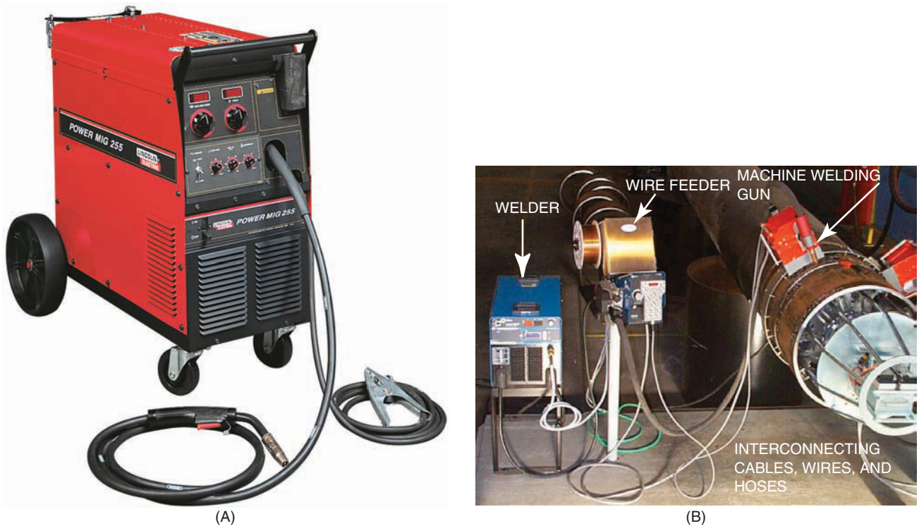
Figure 2.8 GMAW station setup
