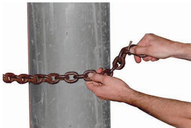
Figure 4.2 Make sure the gas cylinder is chained securely in place before removing the safety cap
