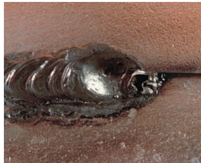
Figure 4.34 Watch the root of the weld bead to be sure there is complete fusion Source: Courtesy of Larry Jeffus
