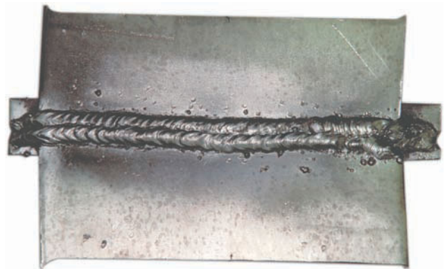
Figure 4.25 Using the ends of a backing strip Run-off tabs, in which the weld starts and stops on the ends of the backing strip, help control possible underfill or burn-back at the starting and stopping points of a groove weld. Source: Courtesy of Larry Jeffus
