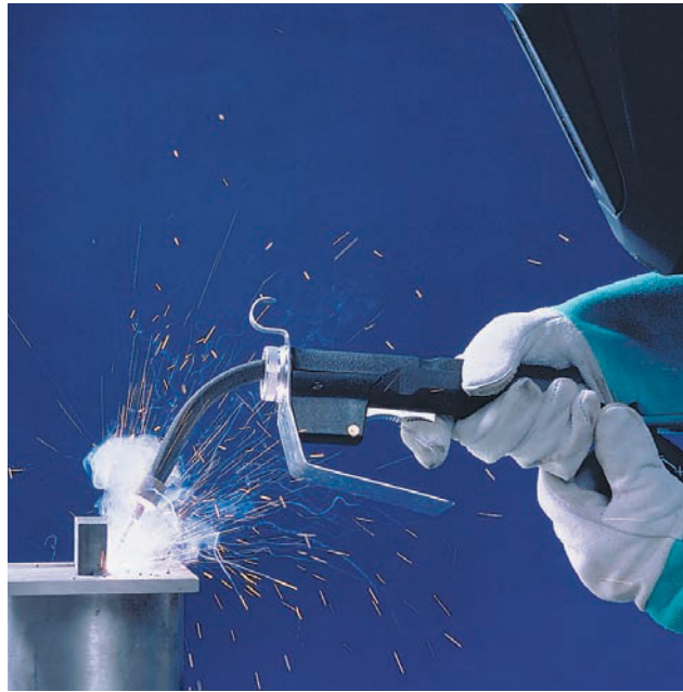
Figure 1.36 A typical GMA welding gun
