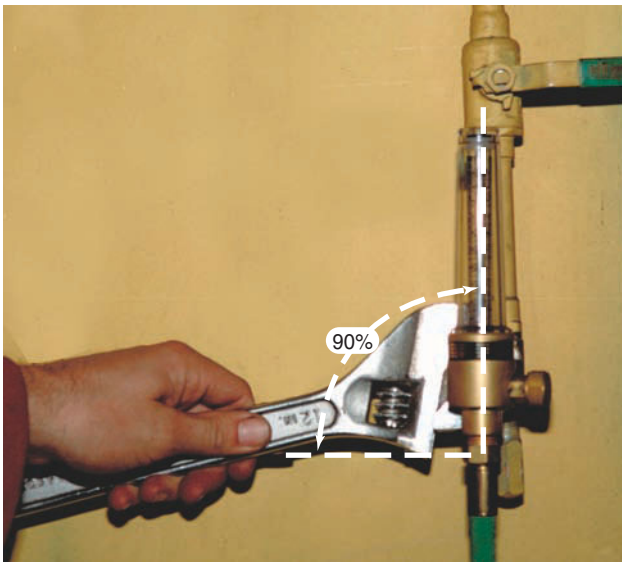
Figure 4.3 Attaching the flowmeter regulator Be sure the tube is vertical. Source: Courtesy of Larry Jeffus
