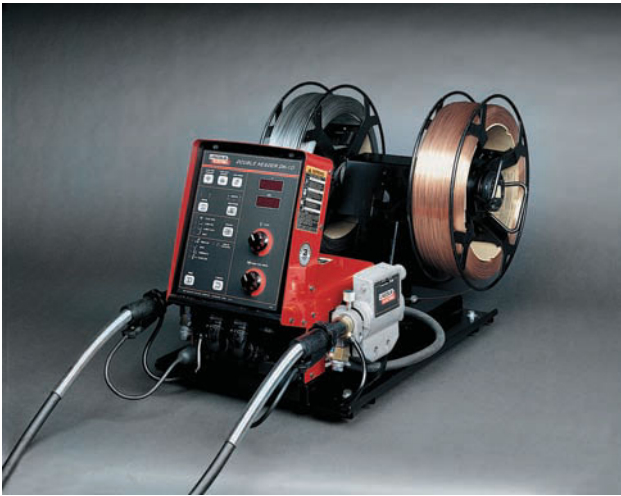
Figure 3.3 Large-capacity wire-feed unit used with FCAW or GMAW
