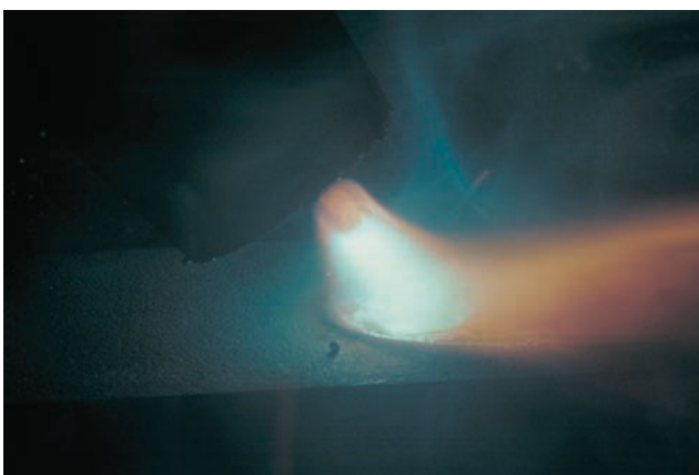
Figure 2.48 GMAW axial spray metal transfer
