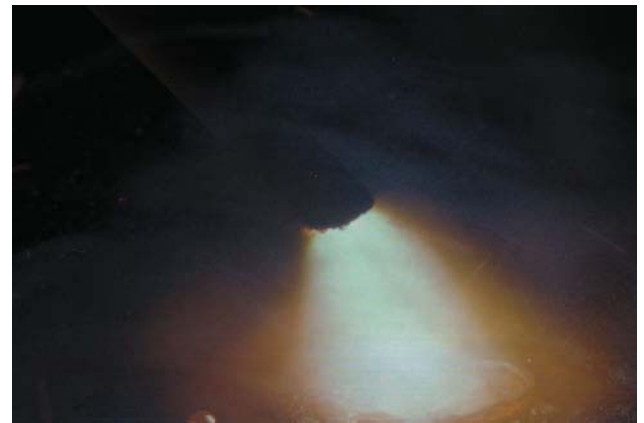
Figure 2.11 Welding with too long an arc length Courtesy of Larry Jeffus
