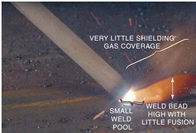
Figure 2.5 Welding with the amperage set too low Courtesy of Larry Jeffus
