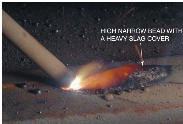
Figure 2.10 Welding with too short an arc length Courtesy of Larry Jeffus
