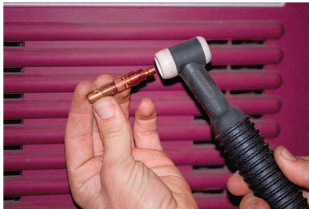
Figure 4.50 Install the nozzle (cup) to the torch body Courtesy of Larry Jeffus
