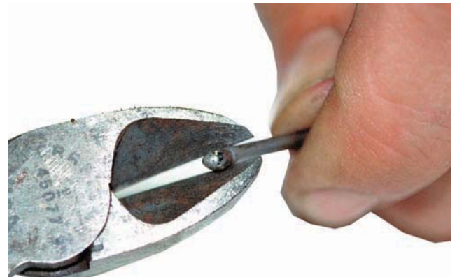
Figure 4.11 Using wire cutters to correctly break the tungsten Courtesy of Larry Jeffus
