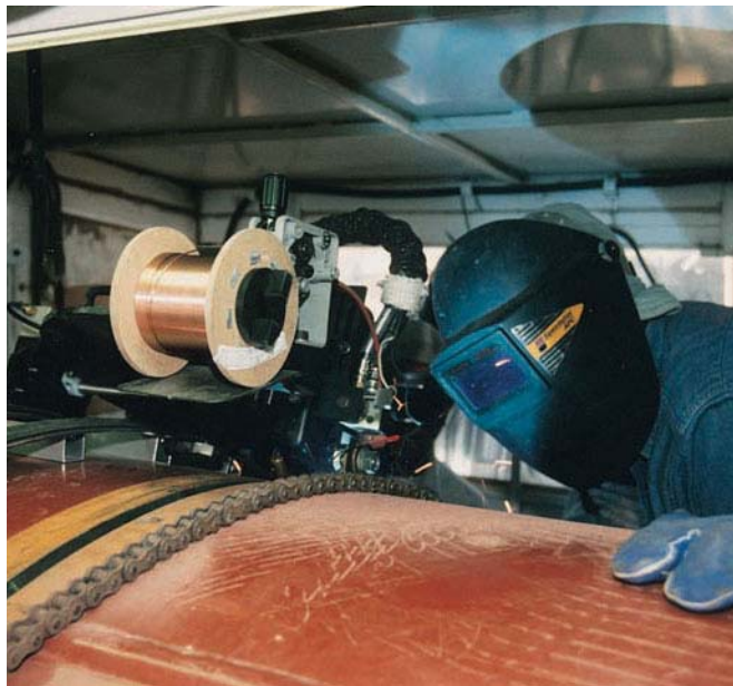
Figure 4.15 Semiautomatic operation allows a stainless steel part to be GTA welded as it is turned past the torch Courtesy of Lincoln Electric Company
