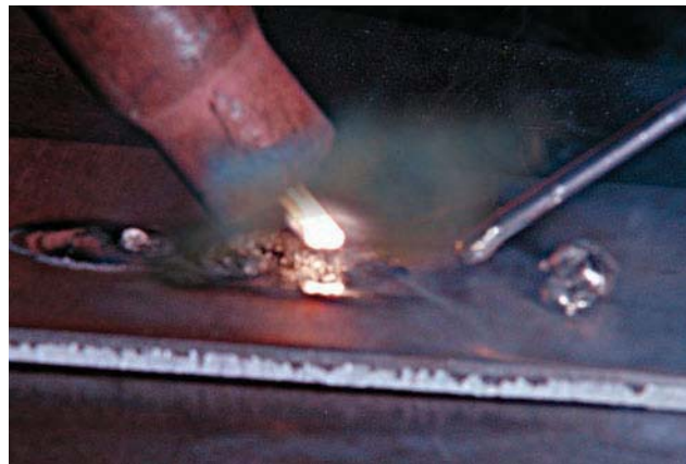
Figure 5.8 Contaminated tungsten Courtesy of Larry Jeffus
