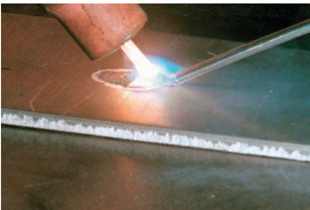
Figure 5.15 Aluminum filler being correctly added to the molten weld pool Courtesy of Larry Jeffus
