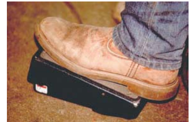
Figure 4.40 A foot-operated device can be used to increase the current Courtesy of Larry Jeffus
