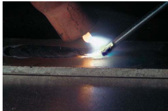
Figure 5.7 Too much filler rod angle has caused oxides to be formed on the filler rod end Courtesy of Larry Jeffus
