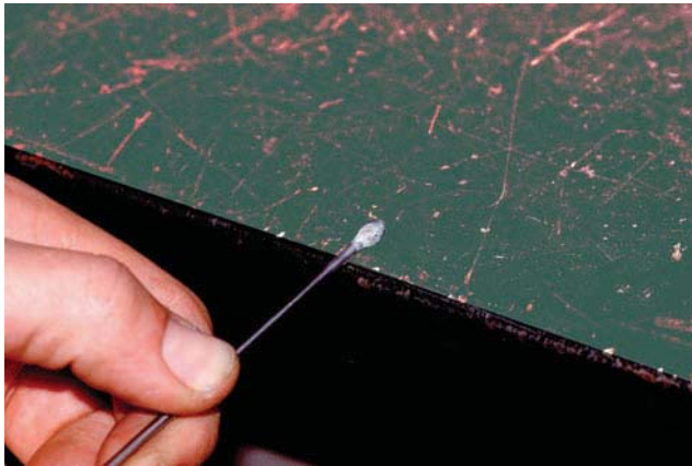
Figure 4.9 Breaking the contaminated end from a tungsten by striking it with a hammer Courtesy of Larry Jeffus
