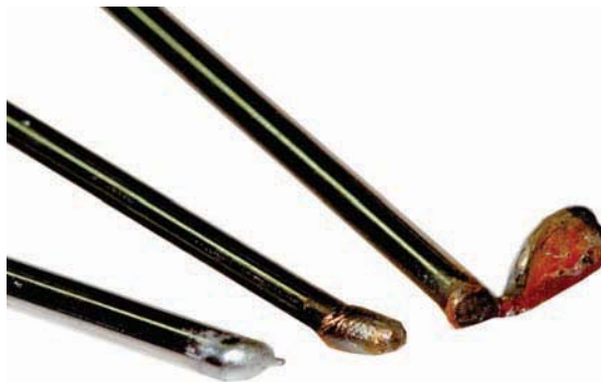
Figure 5.3 (A) Filler properly protected, (B) some oxides on filler, and (C) excessive oxides caused by improper filler rod manipulation Courtesy of Larry Jeffus
