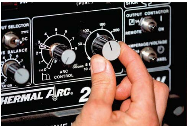
Figure 5.9 Lower the welding current to zero or as low as possible Courtesy of Larry Jeffus
