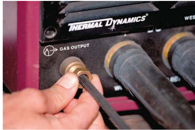
Figure 4.43 Tighten each fitting as it is connected to avoid missing a connection Courtesy of Larry Jeffus
