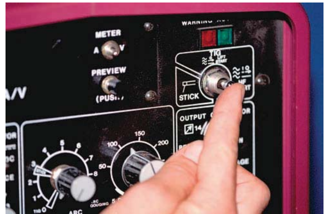
Figure 4.47 The high-frequency switch should be placed in the appropriate position Courtesy of Larry Jeffus
