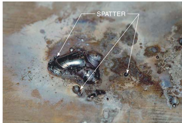
Figure 2.7 Hard weld spatter is fused to base metal and is difficult to remove Courtesy of Larry Jeffus
