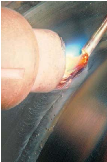
Figure 5.2 The hot filler rod end is well within the protective gas envelope Courtesy of Larry Jeffus
