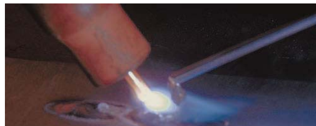
Figure 5.16 Filler rod being melted before it is added to the molten pool Courtesy of Larry Jeffus
