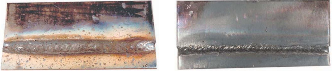
Figure 2.8 Weld before cleaning and after cleaning Courtesy of Larry Jeffus
