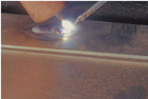
Figure 5.21 Note the difference in the weld produced when different size filler rods are used Courtesy of Larry Jeffus
