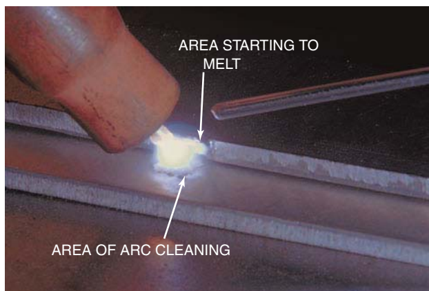
Figure 5.34 Be sure both the top and bottom pieces are melted before adding filler metal Courtesy of Larry Jeffus
