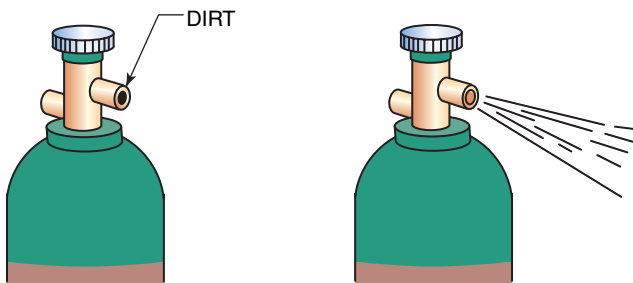
Figure 4.44 During transportation or storage, dirt may collect in the valve. Cracking the valve is the best way to remove any dirt.
