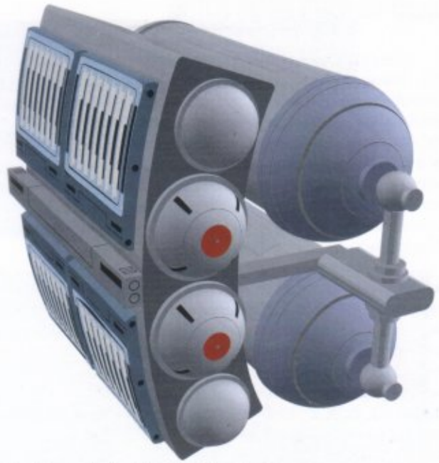
Reaction control systems (RCS) package
