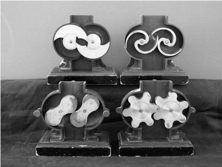
Figure II.35. Reuleaux rotary engine models (Cornell Collection of Kinematic Mechanisms)
