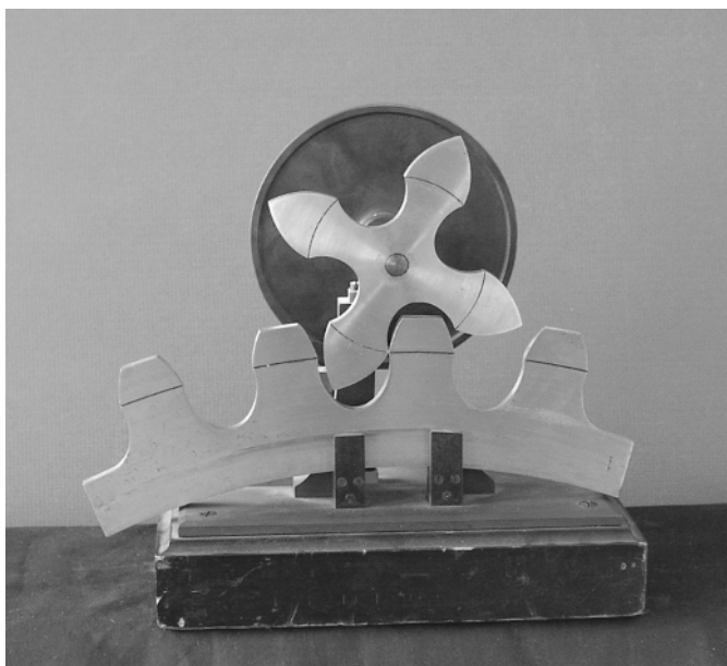
Figure III.13b. Involute spur gear teeth: Reuleaux–Voigt Catalog, Model Q-2 (Cornell Collection of Kinematic Mechanisms)
