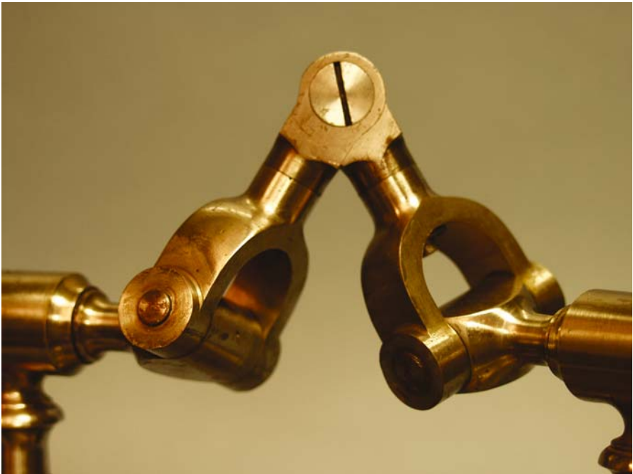
Color Plate 2. Clemen's universal joint coupling. Reuleaux–Voigt Model P-3, Cornell University Collection of Kinematic Models, nickel-plated brass and cast iron, Berlin, circa 1882 (Photo, F.C. Moon)
