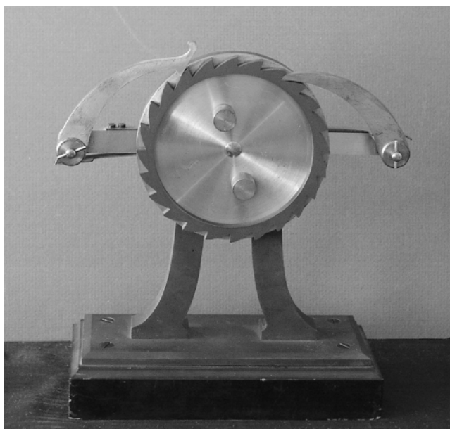
Figure III.11b. Ratchet and Pawl Mechanism: Reuleaux–Voigt Catalog, Model N-17 (Cornell Collection of Kinematic Mechanisms)
