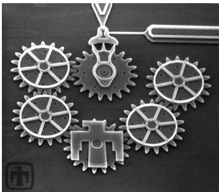
Figure I.8. Micro-electromechanical System [MEMS] gear train; Courtesy: Sandia National Laboratory
