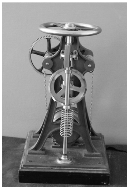
Figure III.12b. Verge and balance wheel escapement: Reuleaux–Voigt Catalog, Model X-1 (Cornell Collection of Kinematic Mechanisms)
