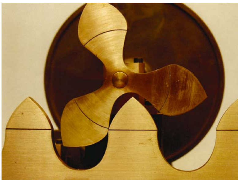
Color Plate 10. Close-up of gear teeth for rack and pinion mechanism. Reuleaux–Voigt Model Q-1, Cornell University Collection of Kinematic Models, nickel-plated brass and cast iron, Berlin, circa 1882 (Photo, F.C. Moon)
