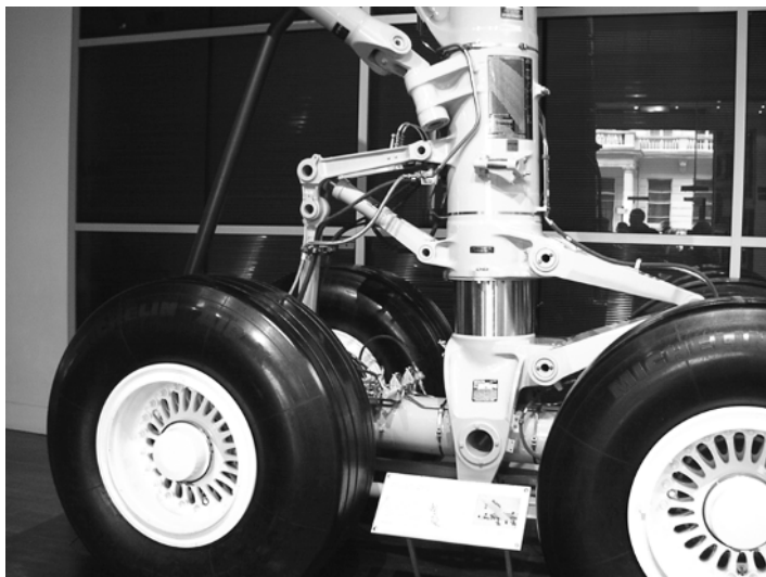
Figure I.7. Landing gear linkage for an Airbus jet. (Science Museum, London)
