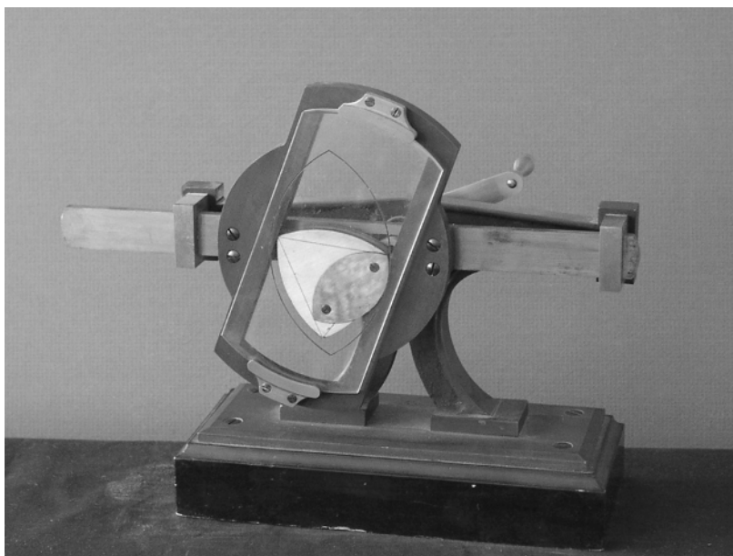
Figure III.18b. Positive-return cam with Reuleaux triangle: Reuleaux–Voigt Catalog, Model L-2 (Cornell Collection of Kinematic Mechanisms)
