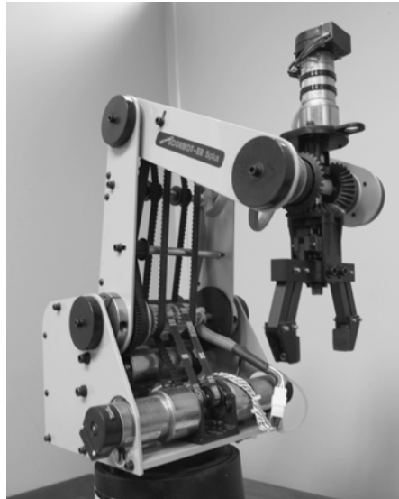
Figure I.9. Modern robotic manipulator arm with end effector gripper
