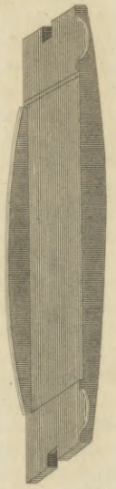
Cast Iron Flat rails Fig. 2.
