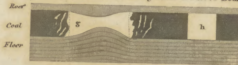
Elevation of the Effect of Driving Broad & Narrow Boards
